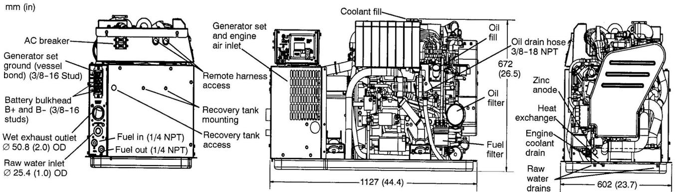
**Note:** This outline drawing is provided for general reference only and is not intended for design or installation. For more information see Operation and Installation manuals or obtain drawing 500-4944 and wiring diagram from your distributor/dealer.
