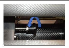
6. Close the reset valve (lever in vertical position).
