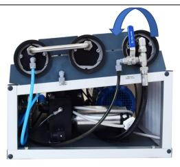
4. Screw the positioner know clockwise until it can be moved no further. Normally 10 turns at least are needed.
