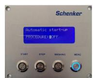
This function activates automatically the first start up procedure. The procedure is necessary when a new machine is started for the first time, or after the filter cartridge replacement, or a general service. The procedure allows to purge completely the air from the system, and from the seawater and the washing fresh water hoses. The depressurization valve <u>must be opened</u> before start the procedure.
