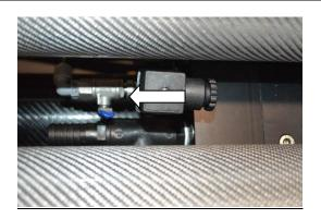
3. Open the depressurization valve at 45°.
