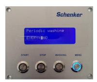
This function allows a periodic automatic rinsing (every 6 up to 10 days) with fresh water. It can be used before long inactivity periods. The single washing operation will last about 1 minute. The consumed fresh water, for every washing, is about 30 liters. Therefore it is suggested to evaluate if the fresh water reservoir is enough for the programmed cycles. Selecting NO, the function will be disabled.
