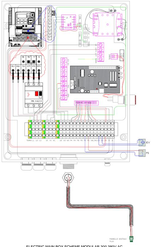
ELECTRIC MAIN BOX SCHEME MODULAR 300 380V AC FIG. 4-6
