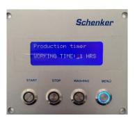
It allows to select the working time of the watermaker (1-6 hours). The timer is activated if the START button is pushed for more than 3 seconds only.
