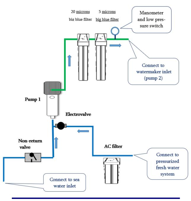
HYDRAULIC CONNECTION AND PIPES FIG. 4-1
