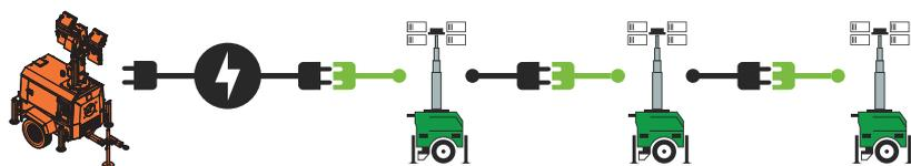
**E' POSSIBILE INOLTRE COLLEGARE 3 LUX C10 IN SERIE AD UNA TORRE CON GRUPPO ELETTROGENA DA 8 KVA**
