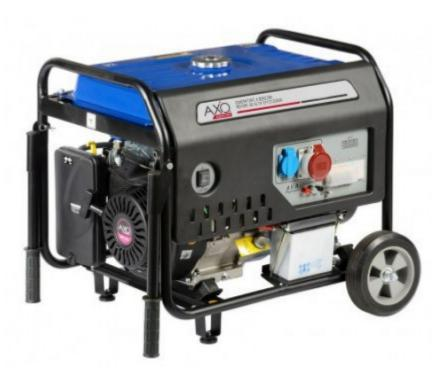
The semi-silent petrol AEGE 6501T generator is equipped with a three-phase alternator with neutral available, THD (total harmonic distortion) value less than 6% and voltage accuracy between +1.5% and -1.5%.
