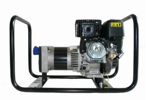
The ACG 5000M petrol generator for worksites is equipped with a single-phase alternator designed and manufactured in Italy. The THD (total harmonic distortion) value is less than 6%, the voltage accuracy is between +5% and -10%.
