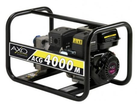
The ACG 4000M current generator for worksites is characterised by a single-phase alternator designed and manufactured in Italy. The THD (total harmonic distortion) value is less than 6%, the voltage accuracy is between +5% and -10%.
