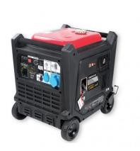
Power supply: Gasoline Starting: Manual / Electric Displacement: 459 cc Voltage: 230 V Frequency: 50 Hz Run time at 50% load: 10. 5 h Tank capacity: 26l Acoustic power: 63 dB(A) @ 7m Automatic voltage regulation: Inverter Length (mm): 730 Width (mm): 610 Height (mm): 730 Dry weight (Kg): 115
