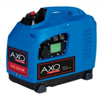
The petrol AIG 1002SM inverter unit is equipped with a multi-phase alternator+ inverter board with stabilised 220V single-phase output. The THD (total harmonic distortion) value is less than 2%, the voltage accuracy is between +1% and -1%.
