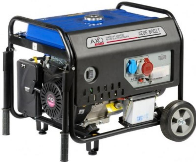
The semi-silent petrol AEGE 8001T generator is equipped with a three-phase alternator with neutral available, THD (total harmonic distortion) value less than 6% and voltage accuracy between +1.5% and -1.5%.
