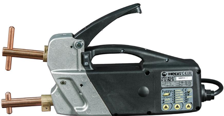
**ENG** • Portable spot-welders which can be directly connected to a grounded power outlet. Designed to be used in demanding applications, the SPOT-WELD is available in two versions: in the first model, spot-welding time is manually controlled by the operator, whereas the second version has electronic time control. The high level of transformer insulation safeguards the operator. Simplicity and low operating costs are the strong points of the SPOT-WELD range.
