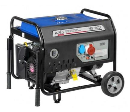
The semi-silent three-phase petrol AEG 5001T generator is equipped with a 3-phase alternator with neutral available, THD (total harmonic distortion) value less than 6% and voltage accuracy between +1.5% and -1.5%.
