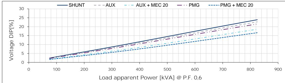
For P.F. different from 0,6 the following simplified formula can be used:  $\Delta V (@ P.F.) = \Delta V (@ 0,6) * \sin(\arccos(P.F.)) / 0,8$
