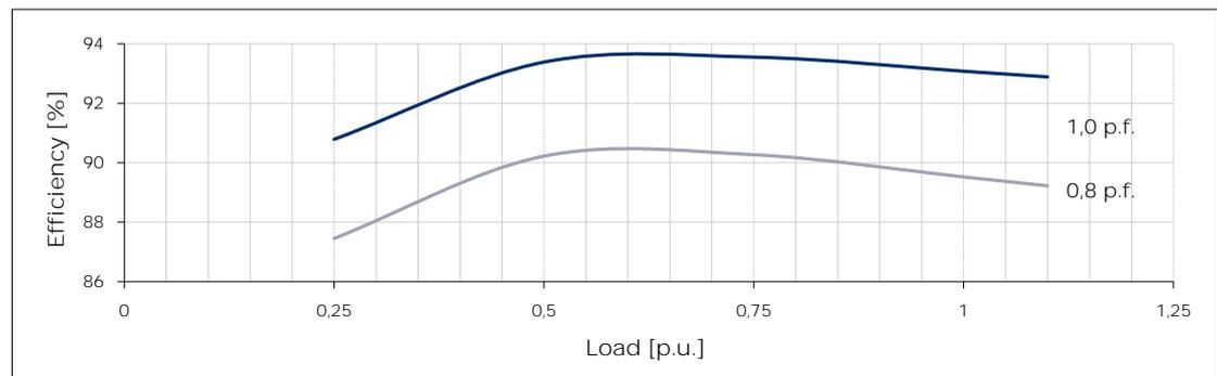
THREE-PHASE SYNCHRONOUS GENERATOR
