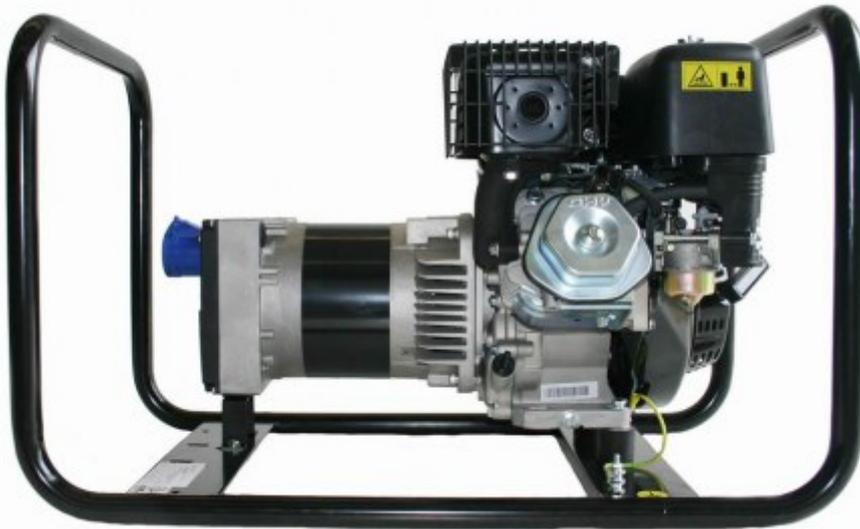
The ACG 5000M petrol generator for worksites is equipped with a single-phase alternator designed and manufactured in Italy. The THD (total harmonic distortion) value is less than 6%, the voltage accuracy is between +5% and -10%.
