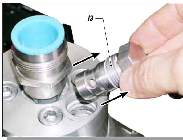
Once it has been cleaned, shake the valve (13) by hand to check that the ball inside moves freely in its seating. If necessary, clean again.
