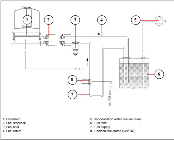
Fig. B.6.1-1: Installation fuel system - example
