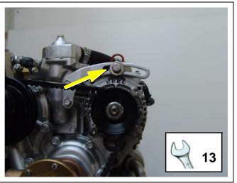
Fig. D.7-1: Fixing screw - DC-alternator
