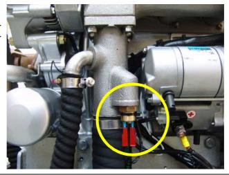
Fig. A.3.7-3: Thermo-switch at exhaust connection
