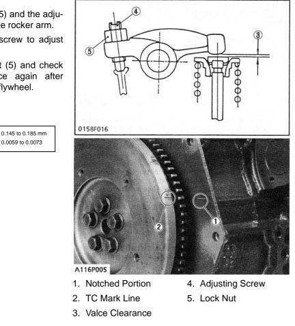
Fig. D.14-1: Valve Clearance
