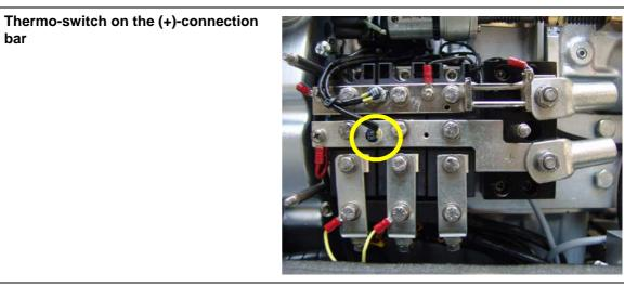
Fig. A.3.7-6: Thermo-switch on the (+)-connection bar
