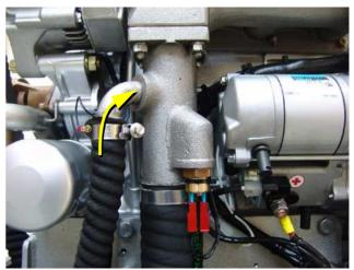
Fig. A.3.2-8: Cooling water injector port
