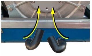
Fig. B.3.5-2: External ventilation valve
