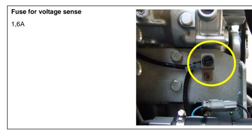
Fig. A.3.6-9: Fuse for voltage sense
