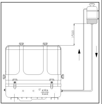
Fig. B.4.1-1: External cooling water expansion tank
