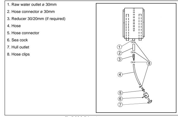
Fig. B.5.2-2: Exhaust/water separator
