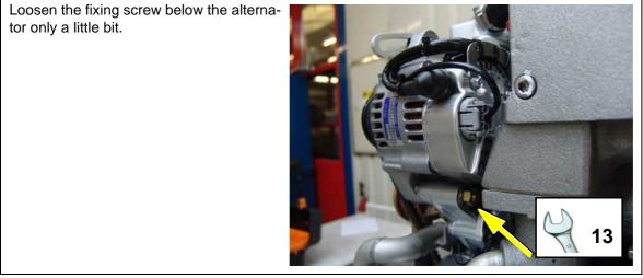
Fig. D.7-3: Fixing screw - DC-alternator
