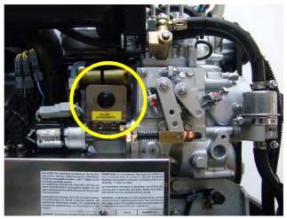
Fig. A.3.7-9: Failure bypass switch
