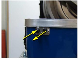
Fig. A.3.3-4: External expansion tank
