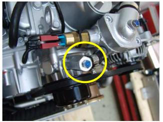
Fig. A.3.3-8: Ventilation screw cooling water pump
