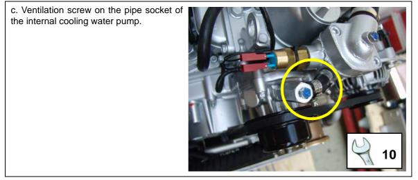
Fig. B.4.2-3: Ventilation screw - water pump
