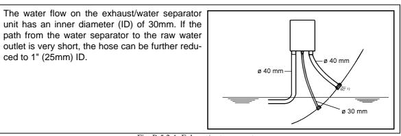
Fig. B.5.2-1: Exhaust/water separator
