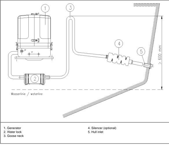
Fig. B.5.1-1: Installation stanrd exhaust system - example
