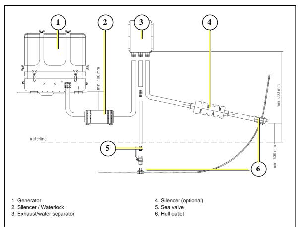
Fig. B.5.3-1: Installation exhaust/water separator - example
