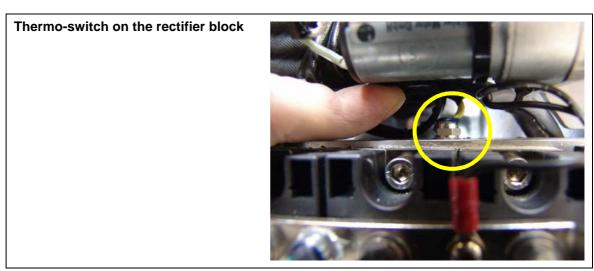
Fig. C.1-7: Thermo-switch on the rectifier block
