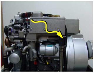
Fig. A.3.3-10: Water-cooled exhaust elbow
