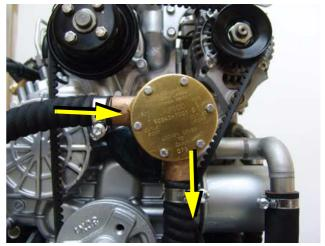
Fig. A.3.2-2: Raw water impeller pump
