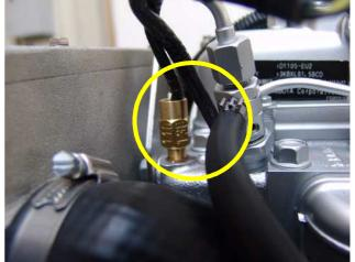
Fig. C.1-1: Thermo-switch at cylinder head
