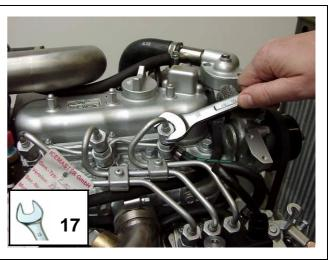
Fig. D.4-3: Injection nozzle
