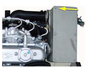
Fig. D.5-1: Air suction housing
