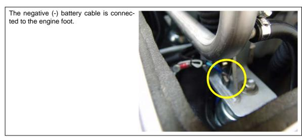
Fig. B.7.1-2: Connection negative battery cable
