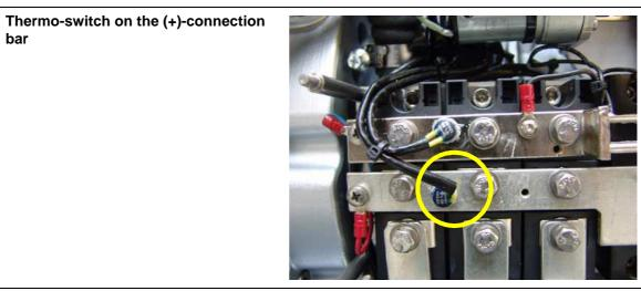
Fig. C.1-6: Thermo-switch on the (+)-connection bar
