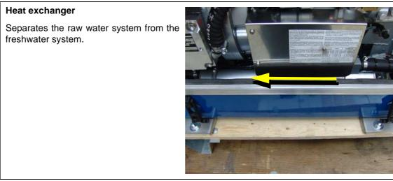
Fig. A.3.2-6: Heat exchanger
