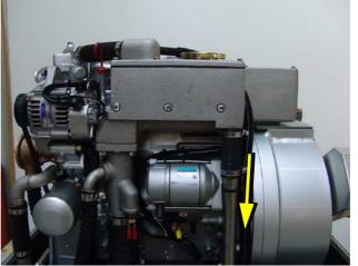
Fig. A.3.3-3: Ventilation pipe
