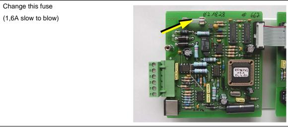
Fig. E.3.2-1: Fuse on VCS board
