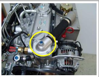
Fig. A.3.3-9: Ventilation screw thermostat housing
