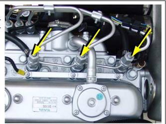
Fig. A.3.4-5: Injection nozzle
