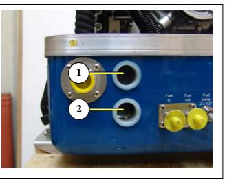
Fig. A.3.6-2: Service battery cables
