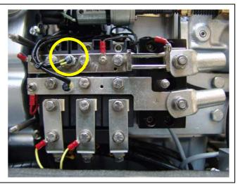
Fig. A.3.7-5: Thermo-switch on the (-)-connection bar
