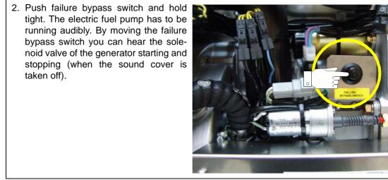
Fig. D.4-1: Failure bypass switch
