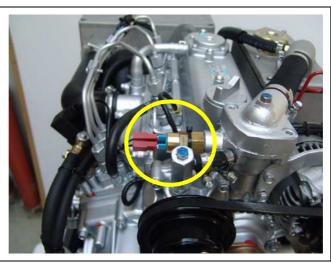
Fig. A.3.7-2: Thermo-switch at exhaust elbow
