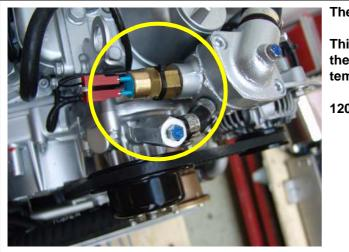
Thermo-switch at thermostat housing
