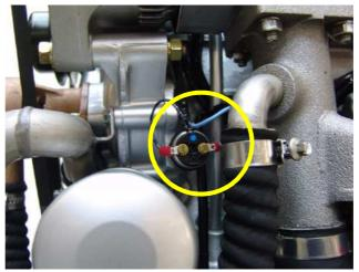
Fig. A.3.7-8: Oil pressure switch
