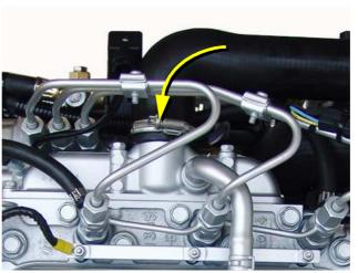
Fig. A.3.5-4: Induction elbow
