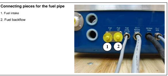
Fig. A.3.4-2: Fuel connections
