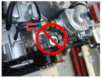
Fig. D.6-5: entilation screw - water pump
