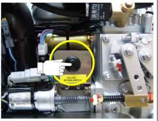
Fig. C.1.3-1: Failure bypass switch
