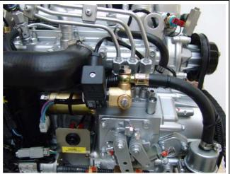
Fig. A.3.4-4: Fuel solenoid valve
