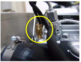
Fig. A.3.7-1: Thermo-switch at cylinder head
