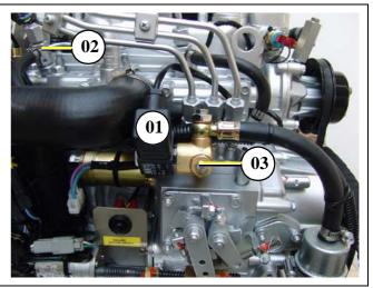
Fig. E.5.2-1: Fuel solenoid valve
