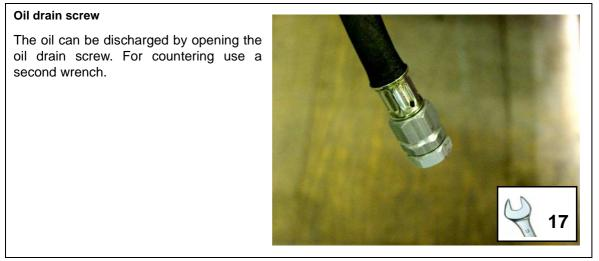
Fig. D.3-2: Oil drain screw
