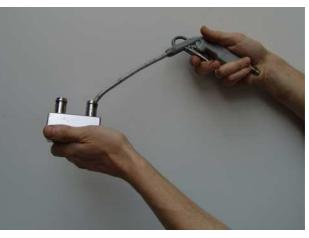
Fig. H.3-9: Cleaning with air
