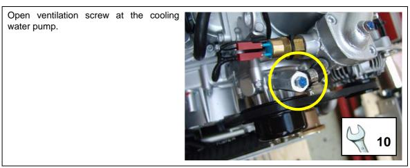
Fig. D.6-2: Ventilation screw - water pump
