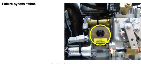
Fig. A.4.5-1: Failure bypass switch
