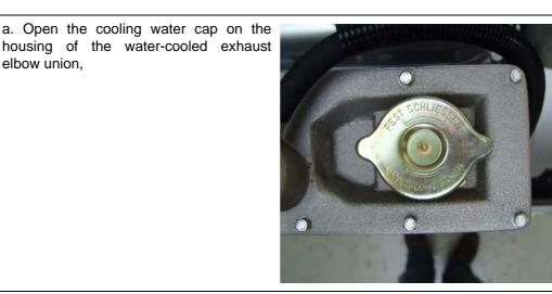
Fig. B.4.2-1: Cooling water filler neck
