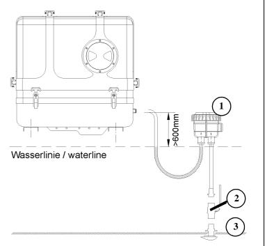
Fig. C.5.0-1: Raw water filter
