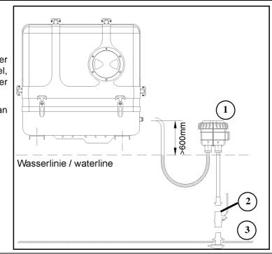
Fig. B.3.4-1: Raw water filter
