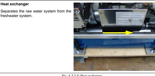
Fig. A.3.3-5: Heat exchanger
