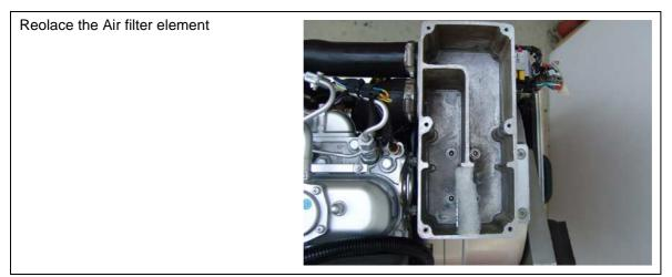
Fig. D.5-2: Air suction housing
