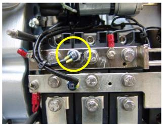
Fig. C.1-5: Thermo-switch on the (-)-connection bar
