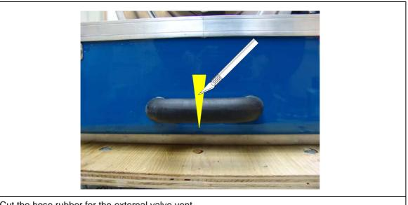
Cut the hose rubber for the external valve vent.....
