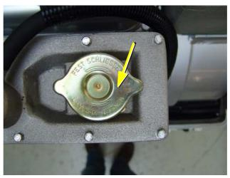
Fig. D.6-4: Cooling water filler neck
