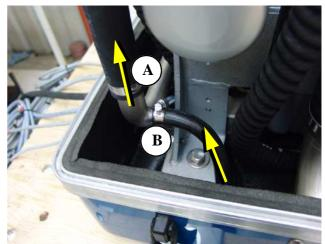
Fig. A.3.3-6: Cooling water injection
