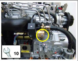
Fig. D.4-2: Ventilation screw - fuel solenoid valve
