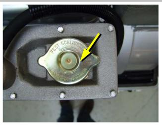
Fig. A.3.3-1: Cooling water filler neck
