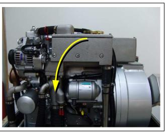
Fig. A.3.5-6: Water-cooled exhaust elbow
