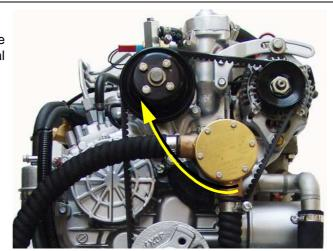
Fig. A.3.3-7: Internal cooling water pump
