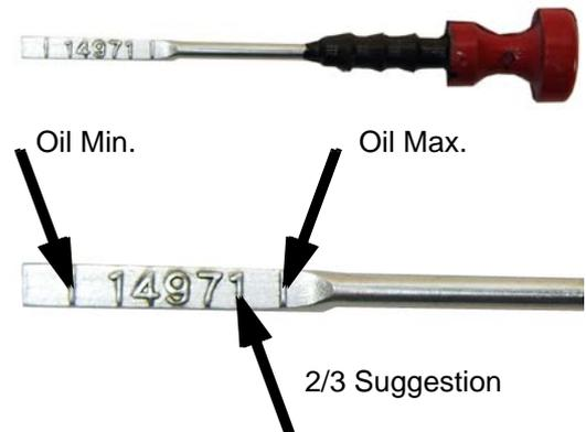
Oil should be refilled, if the oil-level is under 1/3 between the minimum and the maximum mark.
