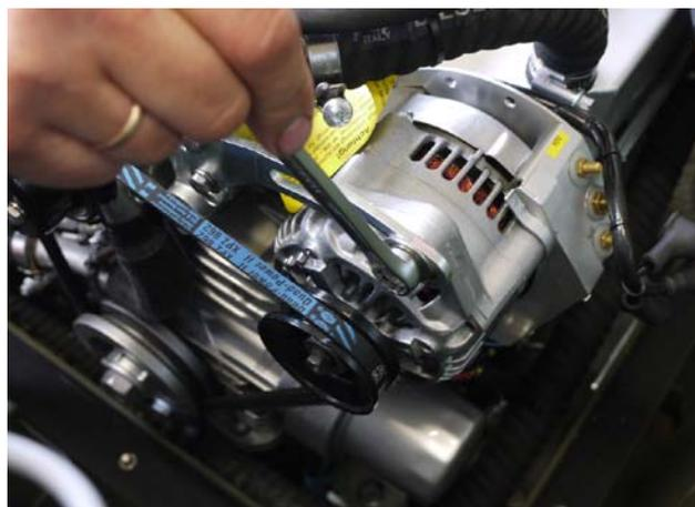
8. Loosen bottom fixing screw of the DC alternator with a wrench with W.A.F. 12 mm (01).
