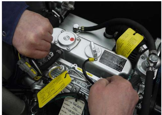
*Fig. 7.29-4: Glow plugs*
