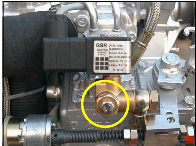
*Not all generator models has a fuel solenoid valve. At generators without fuel solenoid valve, a single ventilation screw is installed.*
