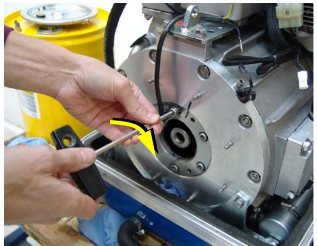
**Mounting the ball bearing:**
