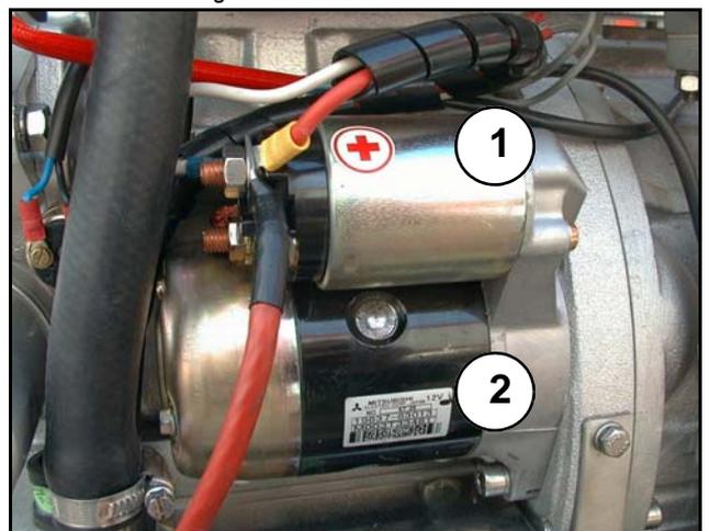
Fig. 6.12.1-4: Connection starterbattery 12V - schema
