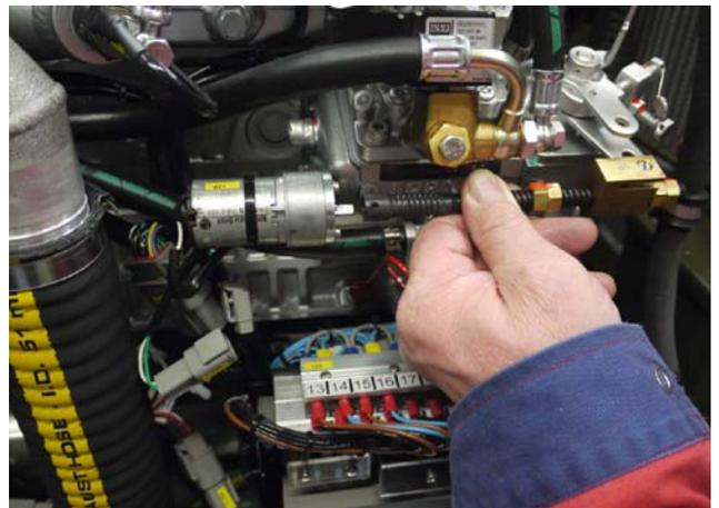
5. Remove screw with a size 0 or 1 screwdriver.
