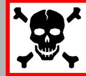
This warning symbol draws attention to special warnings, instructions or procedures which, if not strictly observed, may result in damage or destruction of equipment.
