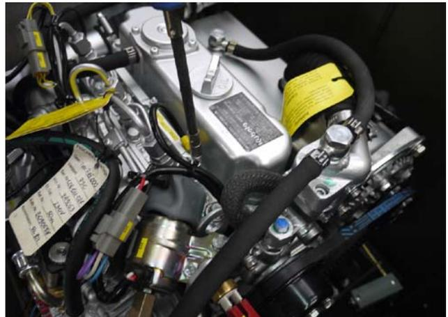
*Fig. 7.29-3: Glow plugs*
