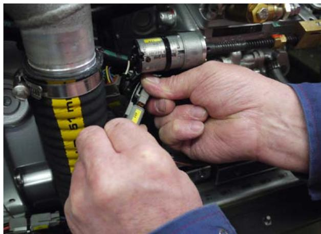
3. Unscrew the grub screw using a size 2 mm socket wrench.
