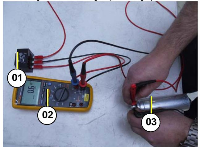
**Discharge the capacitor - three phase**
