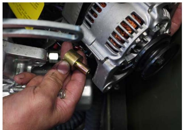
14. Loosen and remove the earthing strip with a size 5 mm socket wrench.
