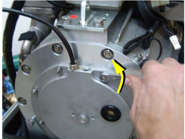
As shown, degrease the spot with a fat solvent and make a mark with a waterproof pen.
