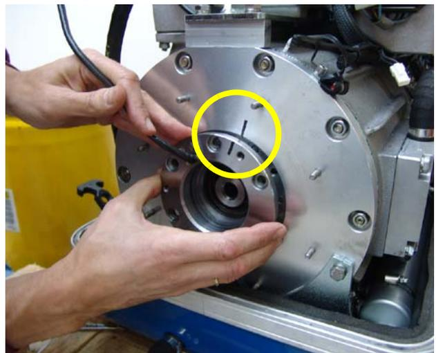
With the other hand, loosely screw in the lifting screws for guidance.
