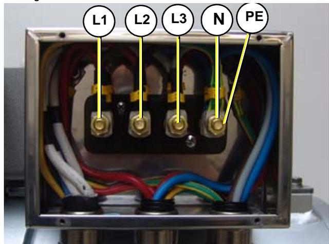
Fig. 8.5.0-4: Wiring diagram HP3 - 400V / 50 Hz
