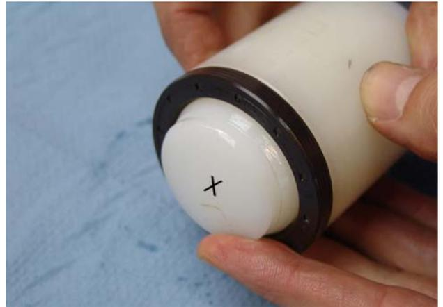
**Mounting of the shaft sealing ring**
