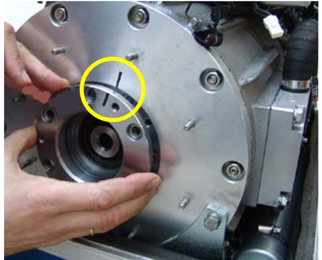
**With the other hand, loosely screw in the ejector screws as guide line.**
