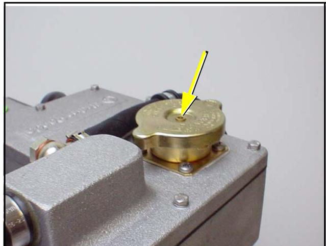
The external compensation tank should be filled to a max 20% in a cold state. It is very important that a larger expansion area is maintained above the cooling water level.
