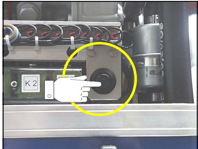
3. Pressing the failure bypass switch for approx 3 - 4 minutes will loosen the ventilation screw located at the fuel solenoid valve. The button must continue to be pressed, whilst opening the screw. A large cloth or Kleenex tissue must be laid beneath the connection to prevent escaping fuel running into the capsule. If the fuel runs out without air bubbles, then the ventilation screw can be closed. Only then may the button be released.
