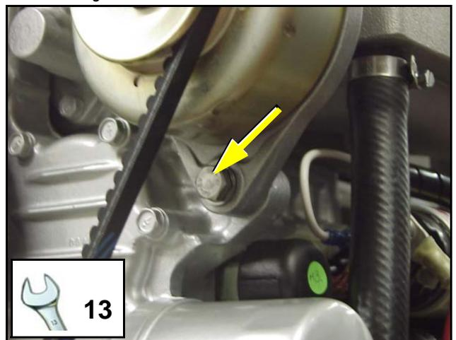
3. The alternator must be pressed in the direction of the thermostat housing.
