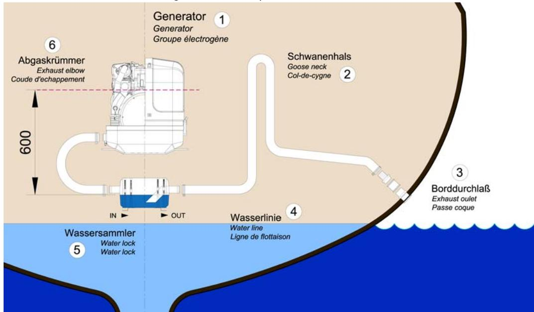
In Fig. 6.8.3.1-1, the waterlock is mounted in center underneath the generator. When the ship tilts, the position of the waterlock related to the critical point at the exhaust hose, changes only slightly.
