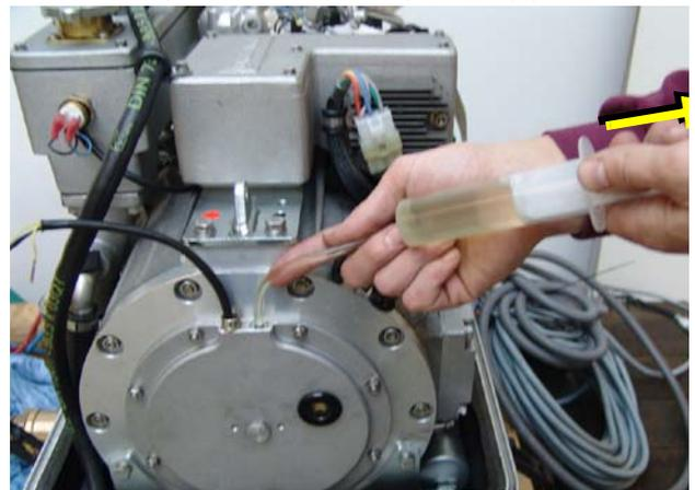
Demount the oil cap by loosening the nuts M6 (Tool: Socket wrench SW10).
