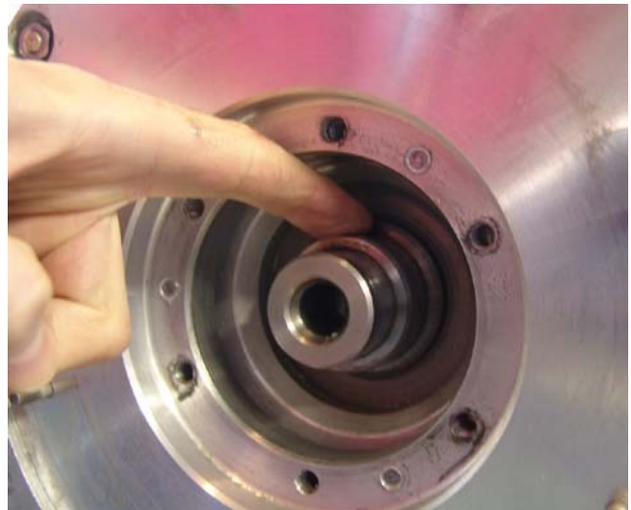
**Mounting the bearing housing inside the generator cap:**
