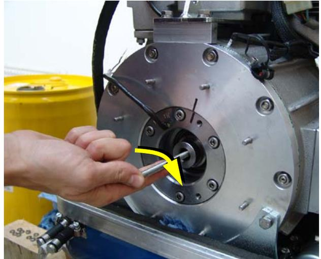
Push the ball bearing, the pressure ladle and the washer up against the shaft, then screw on the hex nuts. Grease/lubricate the thread rod.
