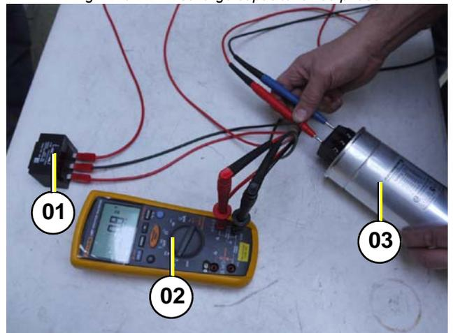
At three phase capacitors the discharge must be made between every phase (L1-L2; L2-L3; L1-L3)
