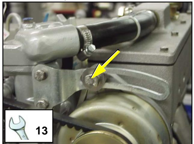
2. Loose the screw underneath the alternator.
