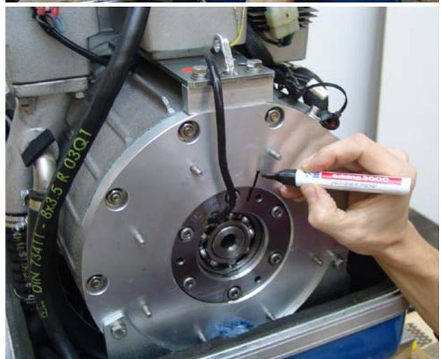
Unscrew the fastening screws (Tool: Allen wrench SW6).
