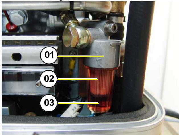
Unscrew the housing from its mount (left hand rotation).
