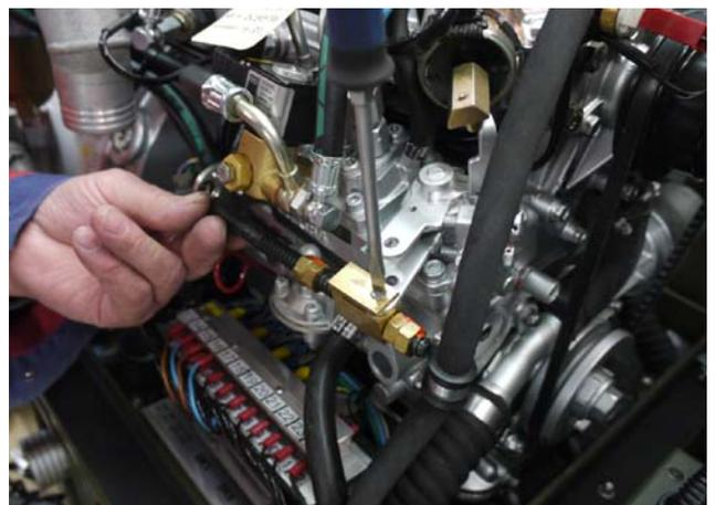
6. Remove the spindle.
