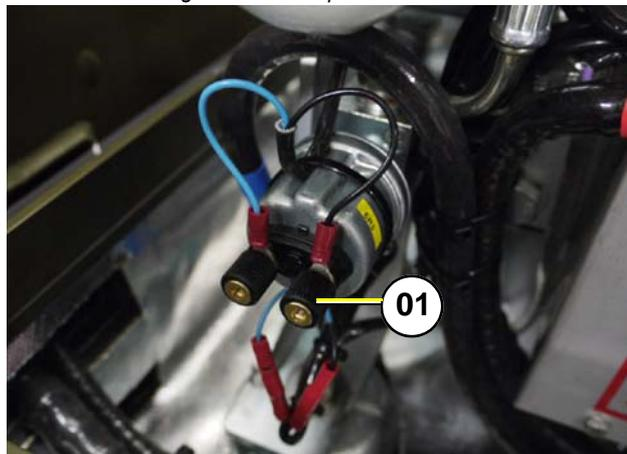
2. Loosen and remove oil pressure sensor 6R3 using a wrench with W.A.F. of 17 mm. A large piece of cloth or absorbent tissue must be placed under the connection to prevent escaping oil from running into the capsule.
