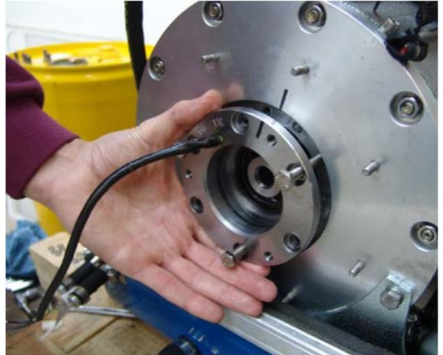
Now carefully press the bearing housing in its seat with a soft headed hammer (or hammer plus mandrel).
