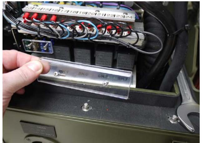
3. Pull relay from the socket and replace with new relay.
