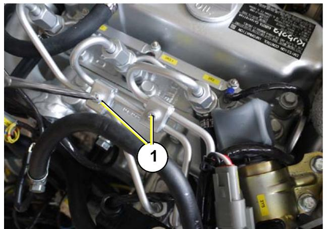
Fig. 7.26-2: Injection nozzles
