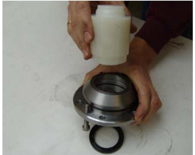
**Remove O-rings from the bearing seat:**
