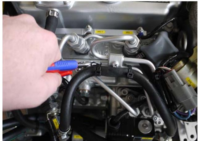
Fig. 7.26-1: Injection nozzles
