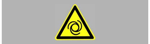
To avoid an unexpected starting of the generator, the starter battery must be disconnected before start working at the generator.
