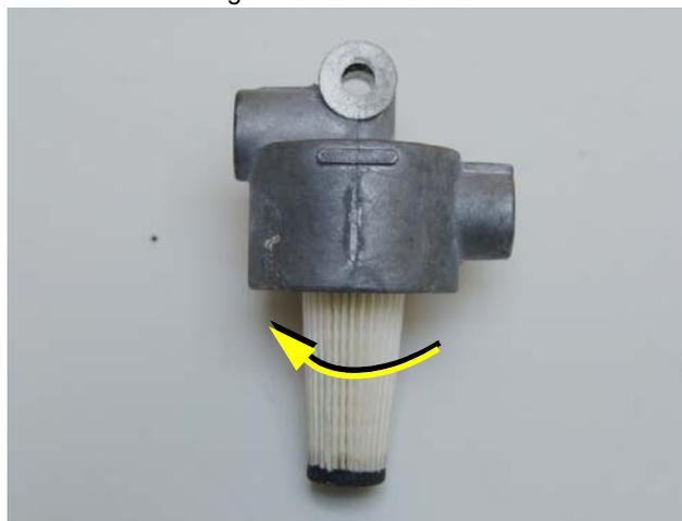
Screw the new filter element into the mount.
