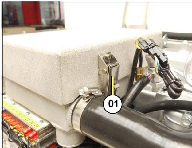
2. Open the combustion air housing by loosening the closure on the left side of the housing.
