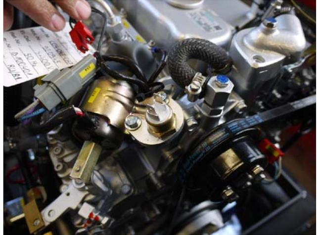
4. Loosen thermostat with a wrench with W.A.F. 22 mm.
