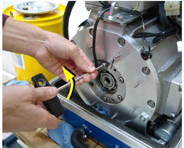
As shown, screw in 3 lifting screws M8x50 as far as possible by hand.
