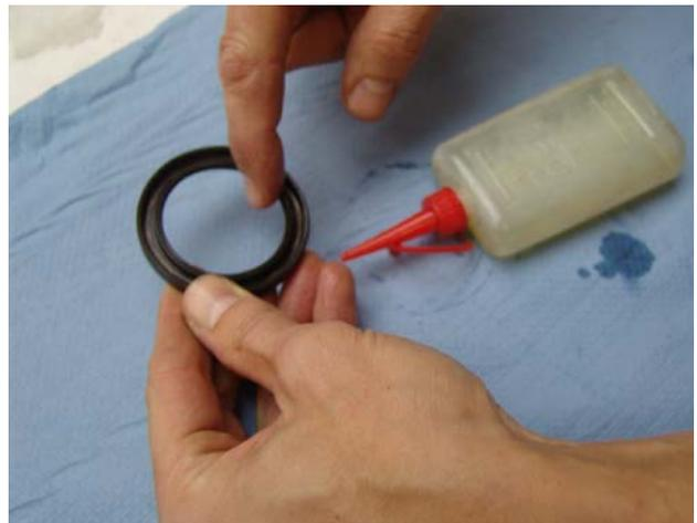
Clean the mandrel, slightly grease/lubricate the connecting surface and the chamber-bevel.
