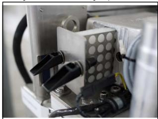
Fig. 7.14.2-3: Air suction housing with pull out holder
