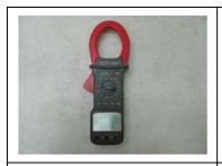
Clamp-on ammeter (DC for synchronous generators; AC for asynchronous generators)
