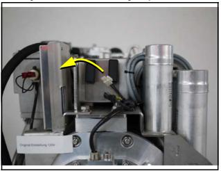
2. Tip the two fasteners 90°.
