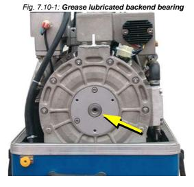
Grease lubricated backend bearing with cooling disc.
