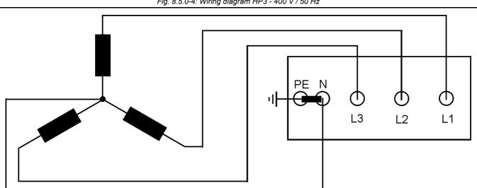
Fig. 8.5.0-4: Wiring diagram HP3 - 400 V / 50 Hz
