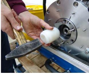
Fig. 7.10.1.3-4: 'Attach bearing case
