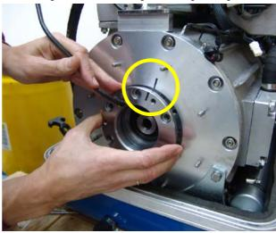
With the other hand, loosely screw in the lifting screws for guidance.
