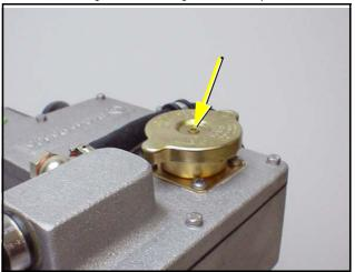
The external compensation tank should be filled to a max 20 % in a cold state. It is very important that a larger expansion area is maintained above the cooling water level.
