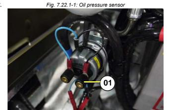
2. Loosen and remove oil pressure sensor 6R3 using a wrench with W.A.F. of 17 mm. A large piece of cloth or absorbent tissue must be placed under the connection to prevent escaping oil from running into the capsule.
