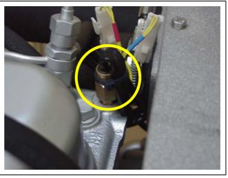
Fig. 4.3.4-1: Thermo-switch at cylinder head
