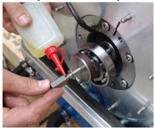
Guide the ball bearing with one hand to avoid canting on the shaft.
