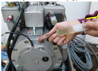
Demount the oil cap by loosening the nuts M6 (Tool: Socket wrench SW10).
