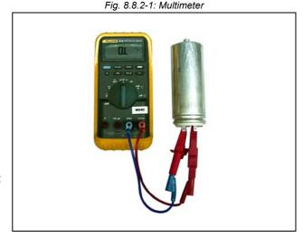
Should a steady sound or no sound be heard, the capacitors are defective and must be replaced.
