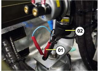
Fig. 7.22-2: Oil pressure sensor
