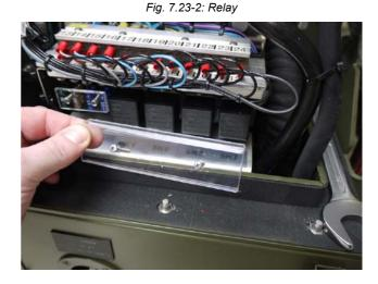
3. Pull relay from the socket and replace with new relay.
