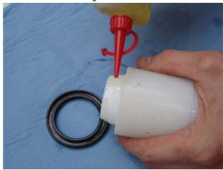
Push the sealing ring on the mandrel, the open side should point towards the handle. The side marked with "X" is to be used.
