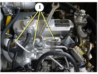
Fig. 7.26-4: Injection nozzles
