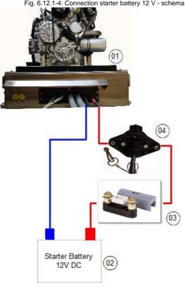
Fig. 6.12.1-4: Connection starter battery 12 V - schema
