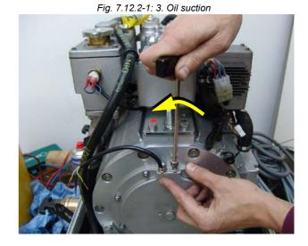
Fig. 7.12.2-2: Oil suction (with syringe)
