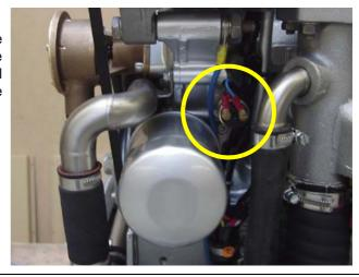
Fig. 4.3.4-5: Oil pressure switch
