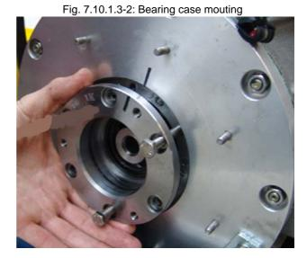
Carefully press the bearing case with a soft-head hammer (or a hammer plus mandrel) in its hub.
