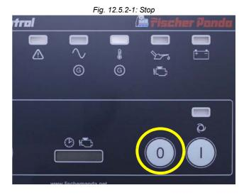
Never switch off the battery until the generator has stopped, if necessary close fuel valve!
