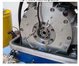
Then screw in those 3 screws with a screw wrench SW13 equally and in turns.
