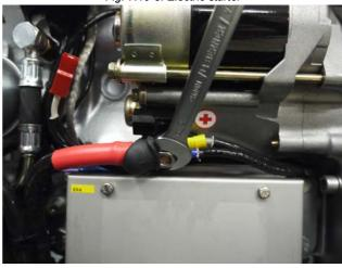
Fig. 7.19-4: Electric starter
