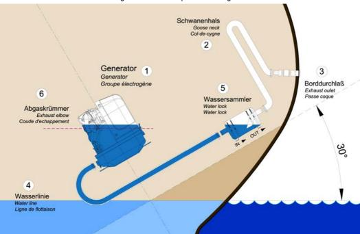
Fig. 6.8.3.2-7: Tilted position 30 degrees
