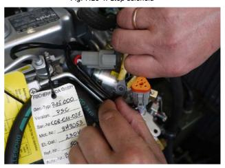
5. Remove the two fixing screws using a size 10 mm socket wrench.
