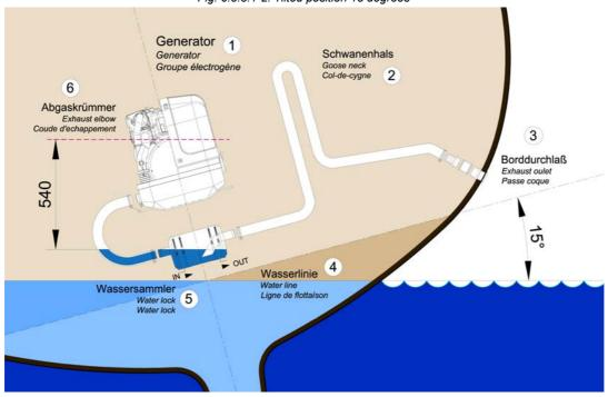
Fig. 6.8.3.1-2: Tilted position 15 degrees
