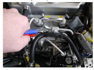
2. Loosen the pipe clamps (1) using a PH2 phillips screwdriver.
