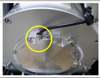
Fig. 4.3.4-4: Thermo-switch at endshield
