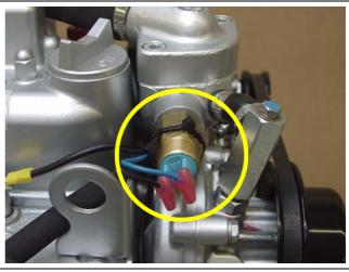
Fig. 4.3.4-2: Thermo-switch at thermostat housing
