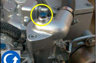
Fig. 7.14-4: Cooling water filler cap
