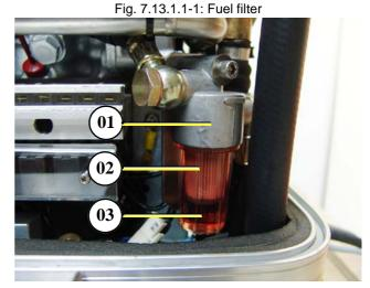
1. Unscrew the housing from its mount (left hand rotation).
