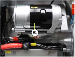
Fig. 7.19-2: Electric starter
