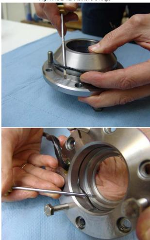
Fig. 7.12.2-13: Remove O-ring
