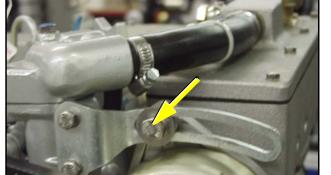
Fig. 7.15-1: Alternator screw
