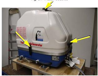
To open the lash closures pull the handle in arrow direction and lift the lash of the closure pin. After lifting of the lashes, the sound isolation cover upper pars can be removed.
