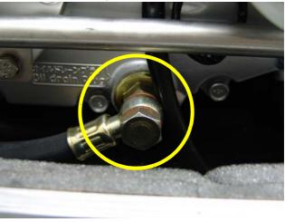
Fig. 7.8-5: Oil screen sealing ring
