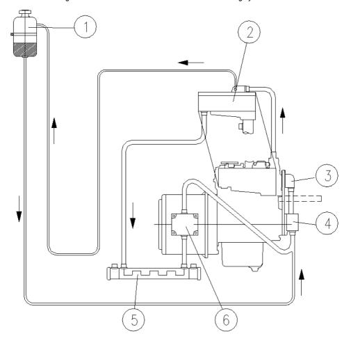
Fig. 6.14.3-1: Fresh water circuit at a two circuit cooling system - Schema
