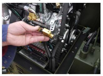
7. Unscrew three screws on the actuator with a size 0 or 1 phillips screwdriver.
