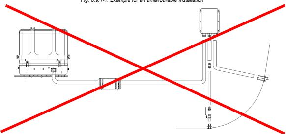
Fig. 6.9.1-1: Example for an unfavourable Installation
