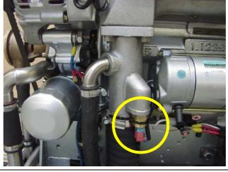
Fig. 4.3.4-3: Thermo-switch at exhaust connection
