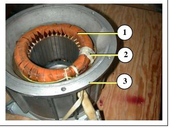
Fig. 4.3.4-6: Thermo-switch coil
