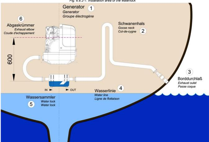
Fig. 6.8.2-1: Installation area of the waterlock
