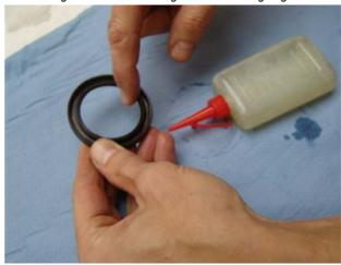
Clean the mandrel, slightly grease/lubricate the connecting surface and the chamber-bevel.
