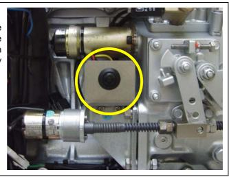
Fig. 4.3.4-7: Failure bypass switch
