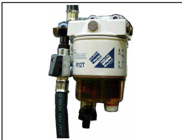
Fig. B.4-1: Pre-filter with water separator
