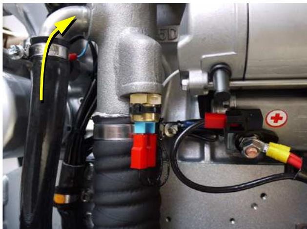
Fig. A.3.2-5: Cooling water injector nozzle
