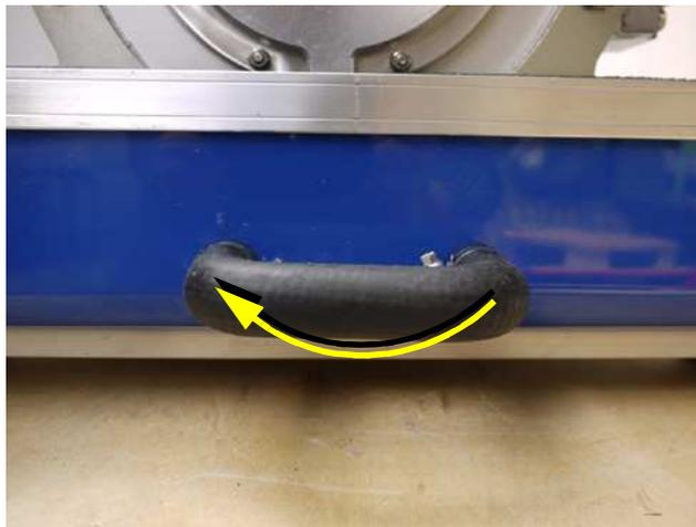
Fig. A.3.2-4: Connection external ventilation valve
