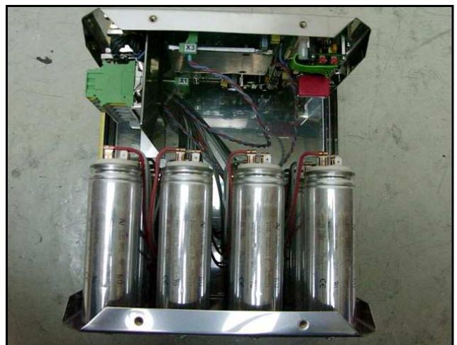
Fig. A.8.3-2: Opened AC Control Box from Panda 30 upwards
