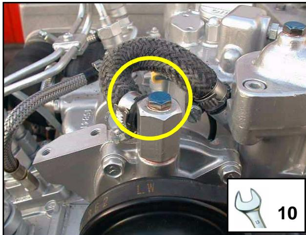
Fig. B.4-2: Ventilating Screw
