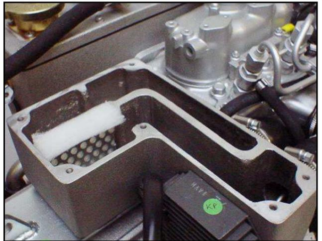
Fig. B.4.3-2: Opened Air Suction Housing
