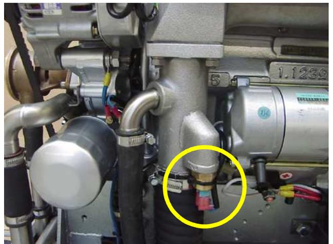
Fig. A.3.7-3: Thermo-switch at exhaust connection
