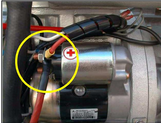
Fig. A.7.1-1: Positive Battery Cable
