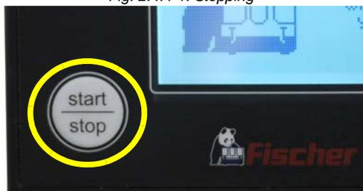
**NOTE:** Never switch off the main battery until the generator has stopped, shut the fuel valve if necessary!
