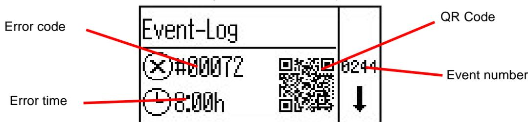
One can scroll through the event memory by using the "Step-up"/"Step-down" keys and then return to the Generator menu with the "Start/Stop - Enter" key.
