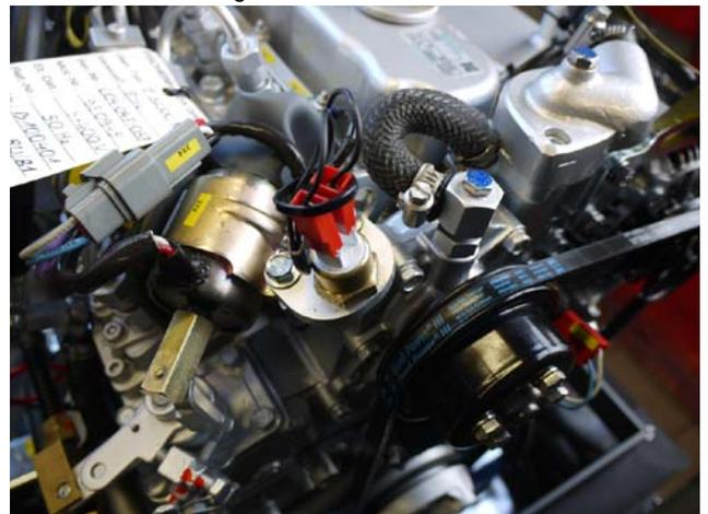
Fig. 6.22-3: Thermocontact
