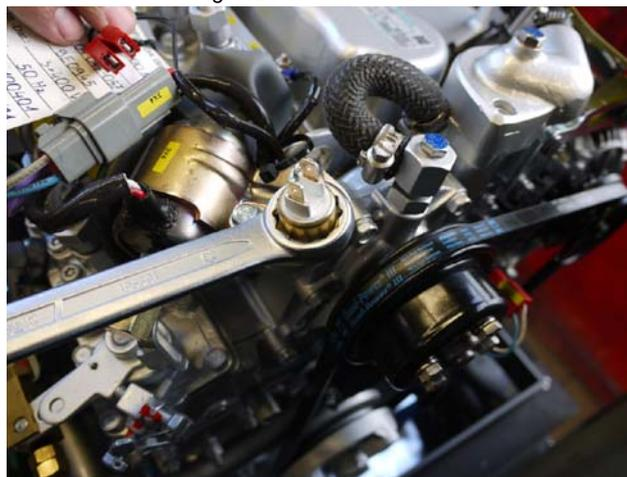
Fig. 6.22-5: Thermocontact
