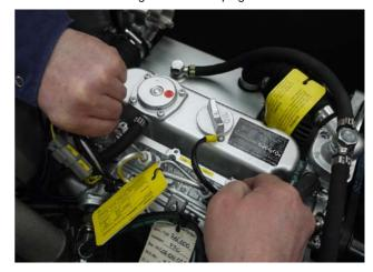
4. Loosen the glow plug using a socket wrench with a long size 10 mm socket.
