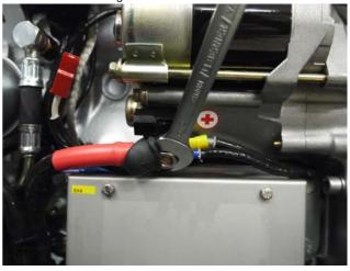
Fig. 7.11-4: Electric starter
