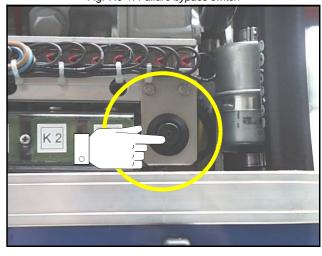
Fig. 7.9-2: Ventilation screw at the fuel solenoid valve
