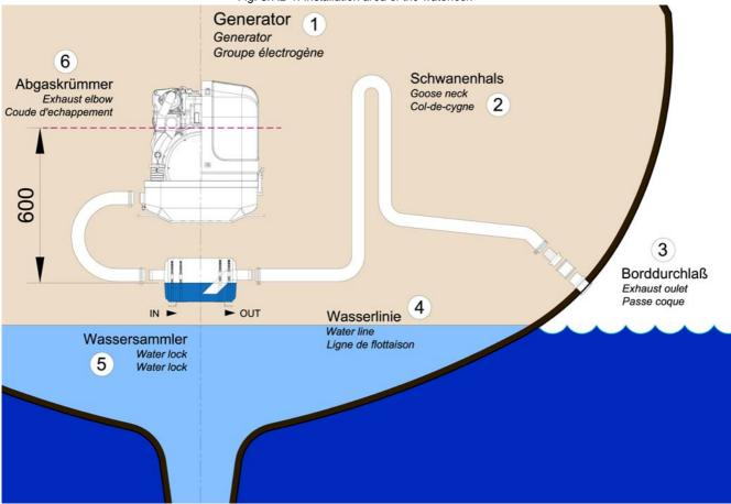
Fig. 5.7.2-1: Installation area of the waterlock
