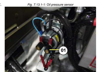
2. Loosen and remove oil pressure sensor 6R3 using a wrench with W.A.F. of 17 mm. A large piece of cloth or absorbent tissue must be placed under the connection to prevent escaping oil from running into the capsule.
