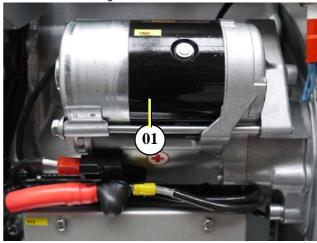
Fig. 7.11-2: Electric starter
