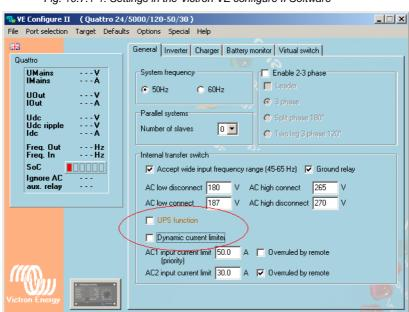
Fig. 10.7.1-1: Settings in the Victron VE configure II Software
