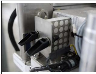
Fig. 7.20.2-4: Air suction housing with pull out holder
