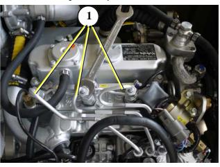
Fig. 7.16-4: Injection nozzles
