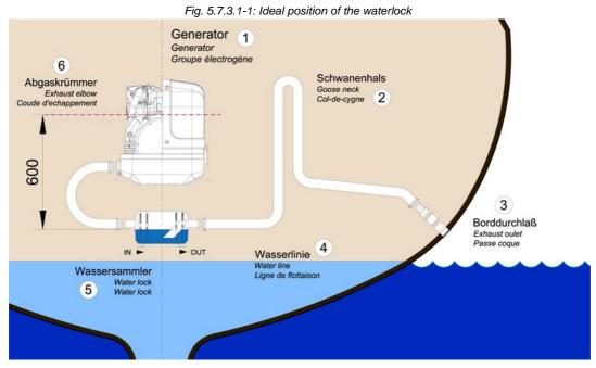
In Fig. 5.7.3.1-1, the waterlock is mounted in center underneath the generator. When the ship tilts, the position of the waterlock related to the critical point at the exhaust hose, changes only slightly.
