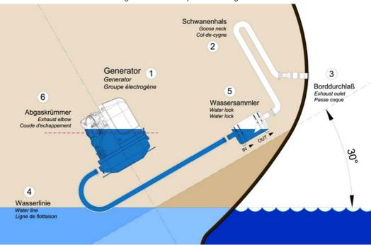
Fig. 5.7.3.2-7: Tilted position 30 degrees
