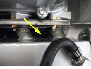
Fig. 7.11-7: Electric starter
