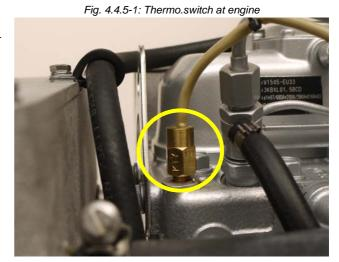
Thermo-sensor at exhaust connection
