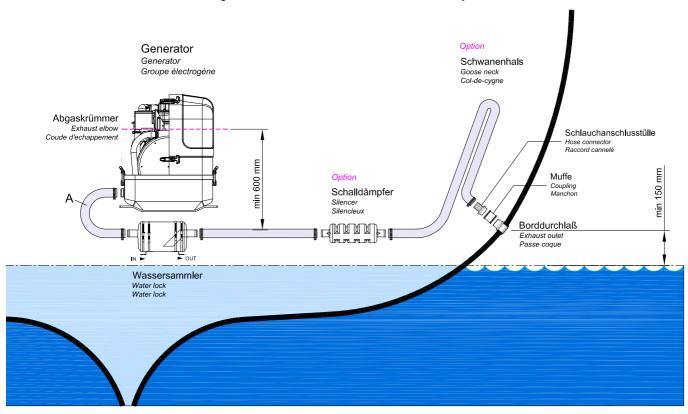
Fig. 5.6.2-1: Installation Scheme Standard Exhaust System
