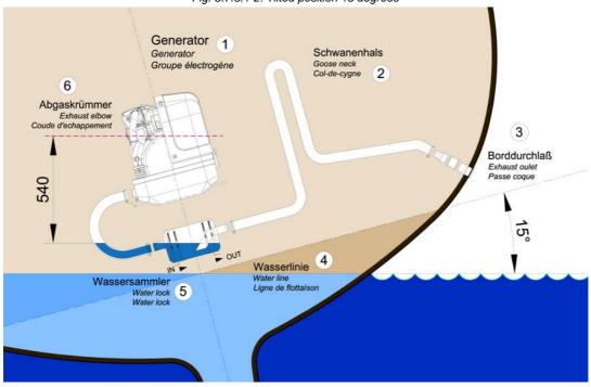
Fig. 5.7.3.1-2: Tilted position 15 degrees
