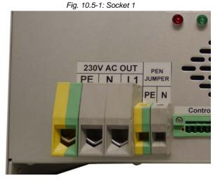
Connecting one of the three Phase with the earth pin will Attention! destroy the PMGi
