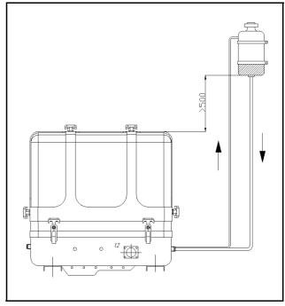
The external cooling water expansion tank may be filled only up to the lower edge of the lower tension tape (see note "max") in the maximum filling level in cold condition.
