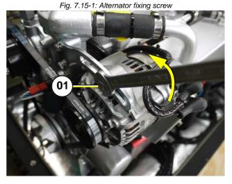
Fig. 7.15-2: Alternator fixing screw
