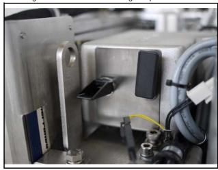
Fig. 7.20.2-3: Air suction housing with pull out holder
