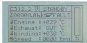
Fault: "Winding", winding temperature too high
