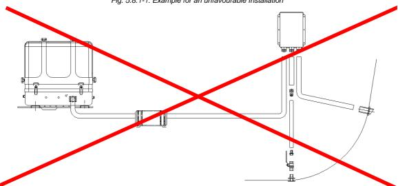
Fig. 5.8.1-1: Example for an unfavourable Installation
