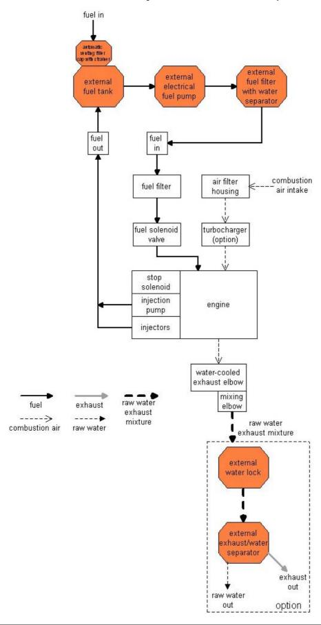
Fig. 4.4.2-1: Fuel, air intake and exhaust system
