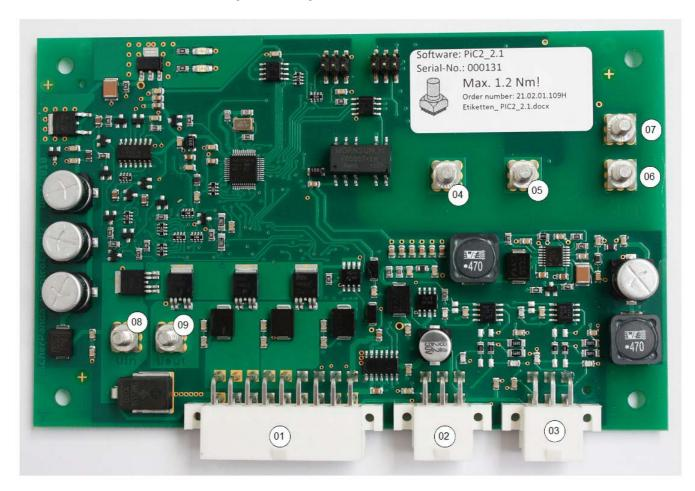
The Panda iControl2 controller is connected to the wire harness with the 18-pin jack. The centre 6-pin jack is designed for the Fischer Panda standard bus. The Panda iControl2 panel is connected to this jack. The Fischer Panda CAN bus is connected to the 6-pin jack at the bottom right of the circuit board. The configuration of the connectors is given in the subsequent tables. Siehe "Terminal assignments on the Panda iControl2 controller" auf Seite 206.
