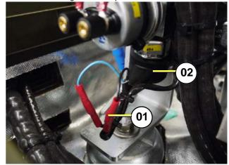
Fig. 7.13-2: Oil pressure sensor
