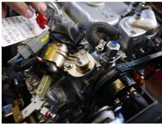
4. Loosen thermoswitch with a wrench with W.A.F. 22 mm.
