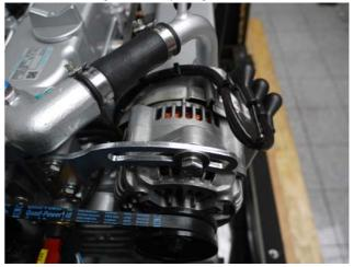
5. The V-belt is tensioned by pulling back the alternator. The V-belt should yield approx. 1 cm when pushed in with a thumb.
