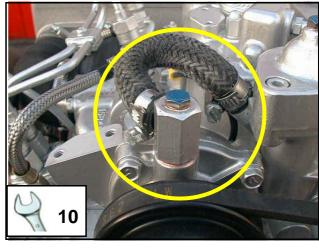
Fig. 7.20.4-3: Venting screw at the thermostat housing
