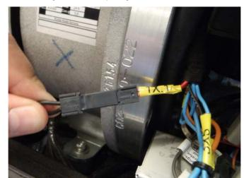
Fig. 2.5-1: Not Stop bridge in the cable harness
