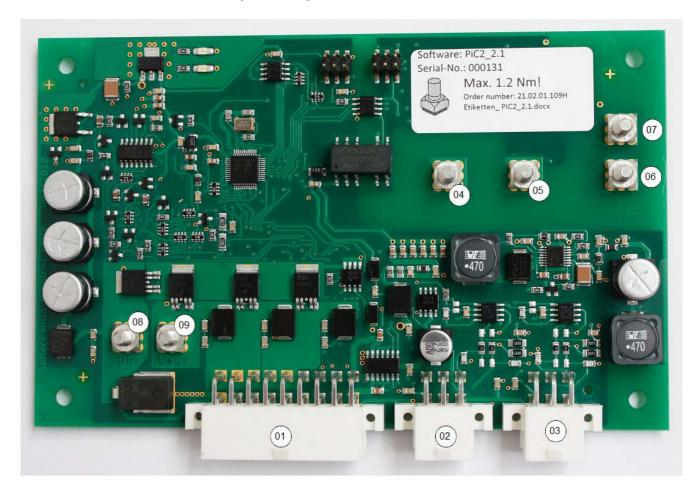
The Panda iControl2 controller is connected to the wire harness with the 18-pin jack. The centre 6-pin jack is designed for the Fischer Panda standard bus. The Panda iControl2 panel is connected to this jack. The Fischer Panda CAN bus is connected to the 6-pin jack at the bottom right of the circuit board. The configuration of the connectors is given in the subsequent tables. Siehe "Terminal assignments on the Panda iControl2 controller" auf Seite 30.
