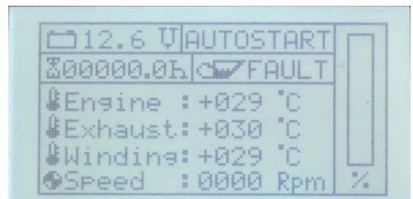
The autostart function will remain active even after the controller is switched off and on again with the On/Off button. To deactivate the autostart function, the flag in the EEPROM must be reset with "Disable". Siehe "Activating/deactivating the autostart function ("Autostart")" auf Seite 19.
