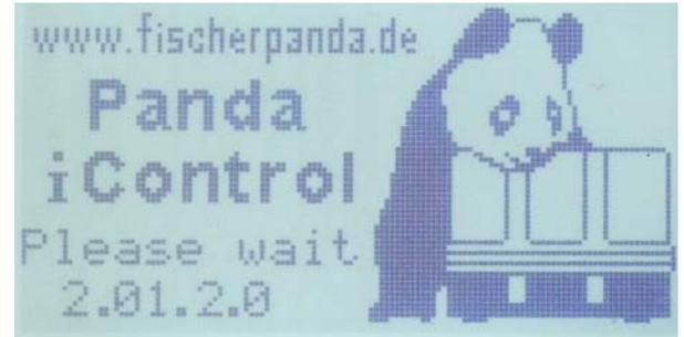
Fig. 2.3.1-2: Hardware version, generator type, and software version in default display
