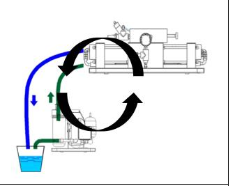
9. Shut the plant off and connect the original hoses.
