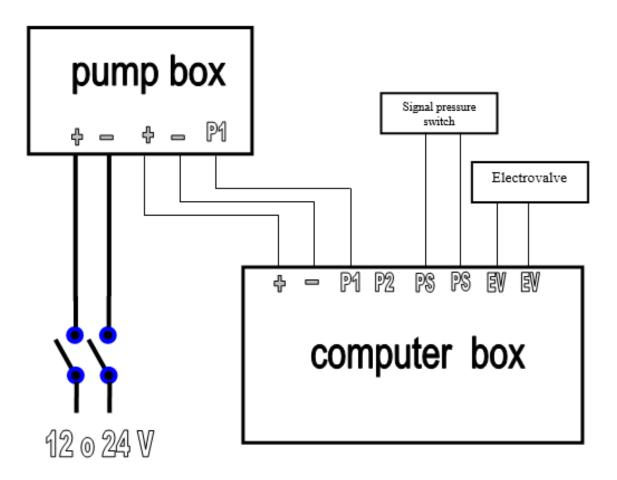
WIRING LOGIC SCHEME12-24 VDC FIG. 4-4
