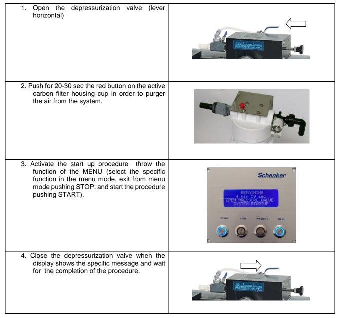
The procedure lasts about 3 minutes, and it can anyway be stopped anytime pushing STOP. After completed the procedure the system is ready to start normally.
