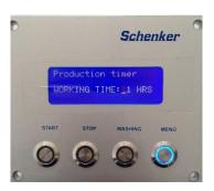
It allows to select the working time of the watermaker (1-6 hours). The timer is activated if the START button is pushed for more than 3 seconds only.
