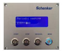
This function allows a periodic automatic rinsing (every 6 up to 10 days) with fresh water. It can be used before long inactivity periods. The single washing operation will last about 1 minute. The consumed fresh water, for every washing, is about 30 liters. Therefore it is suggested to evaluate if the fresh water reservoir is enough for the programmed cycles. Selecting NO, the function will be disabled.
