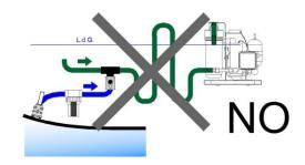
All the hydraulic connections (to exception of the fresh water production) have to be realized with a 16 mm. int. diam. hose and a  $\frac{1}{2}$ " holder. The hydraulic section that is continuously under consistent pressure is the pump outlet -5 m. filter — watermaker inlet connections. For this section is necessary to use a good quality **PN 16 min.** reinforced hose. An inadequate hose could burst, jeopardizing seriously the safety of the boat.
