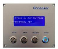
It allows to exclude the sensor (signal pressure switch) that detects the correct cycling of the ERS. The operation with the by-pass is necessary <u>only</u> in case of malfunctioning of the signal pressure switch (in example if the system gets blocks, with the message " SYSTEM BLOCKED", not as consequence of a real hydraulic problem, but just as consequence of the malfunctioning of the probe).
