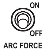
On machines with an Arc Force selector, the same result can be obtained by turning the selector "ON" or "OFF". When switched "ON" a base current is applied to the welding current output acting as a sort of "automatic" arc forcing that does not need to be regulated.
