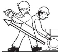
Pull the rope hard and fast. Pull it all the way out. Use two hands if necessary.
