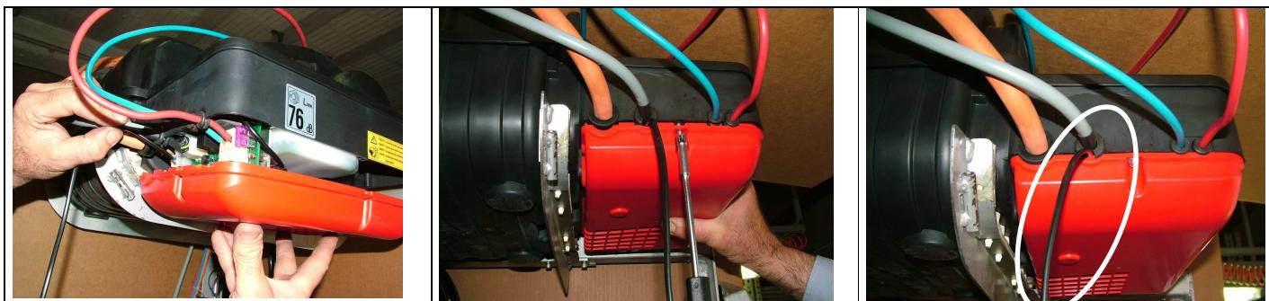
After the test, close the inspection cover of TG480/600.
