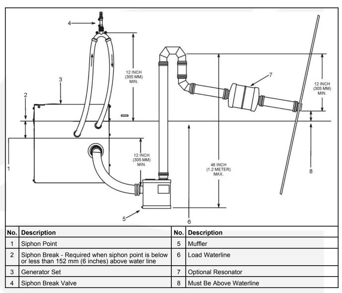
FIGURE 5. TYPICAL WET EXHAUST SYSTEM WITH RESONATOR
