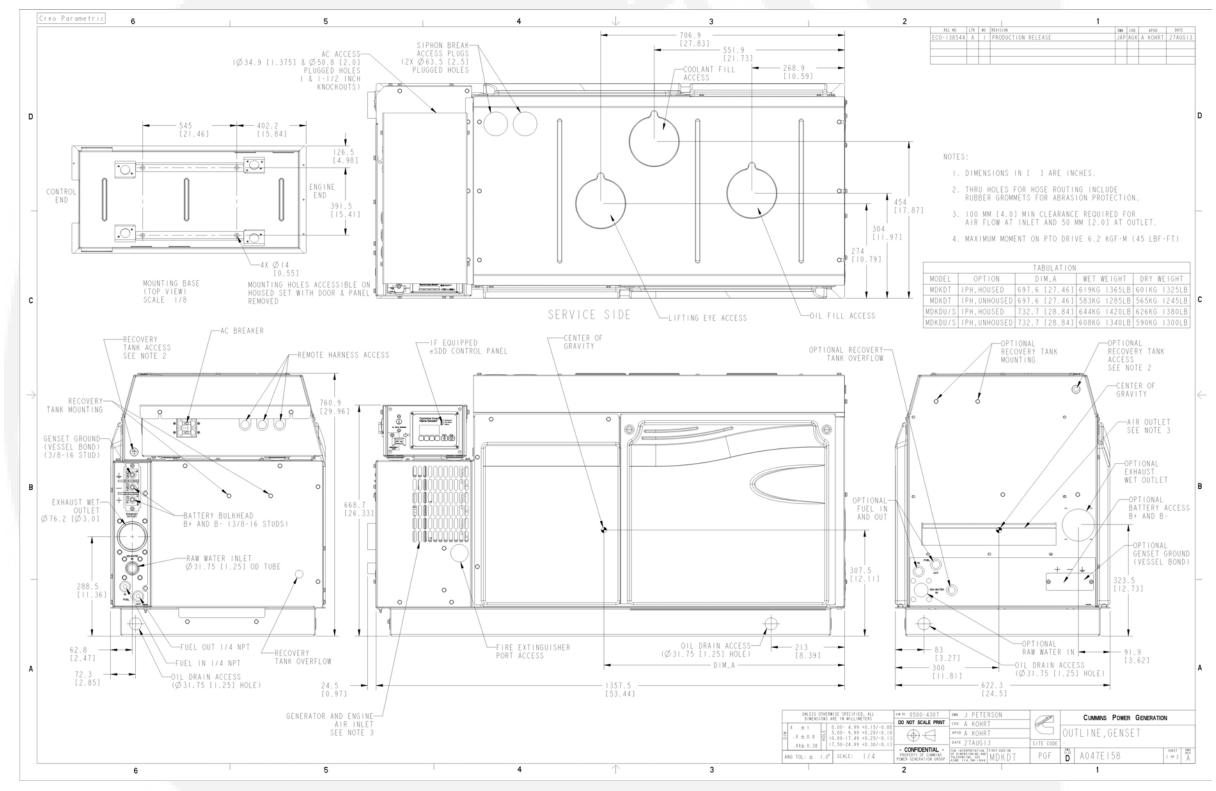
FIGURE 21. MDKDS, MDKDT, MDKDU OUTLINE DRAWING (SHEET 1)
