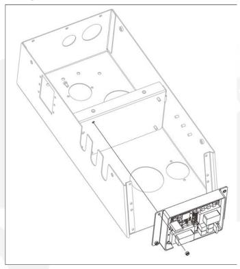
FIGURE 9. NIM MOUNTING LOCATION
