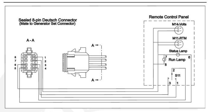
FIGURE 8. CONNECTIONS BETWEEN REMOTE PANEL AND ITS 8-PIN CONNECTOR
