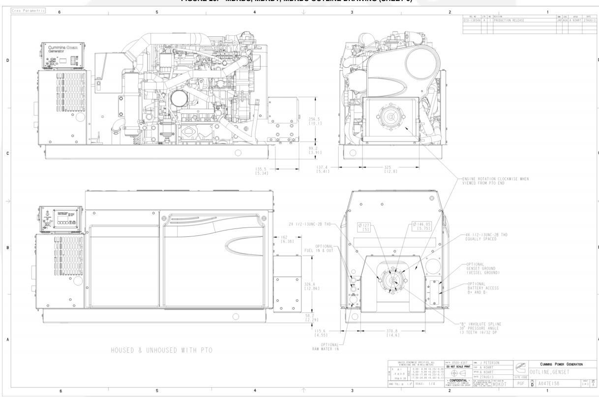
FIGURE 23. MDKDS, MDKDT, MDKDU OUTLINE DRAWING (SHEET 3)
