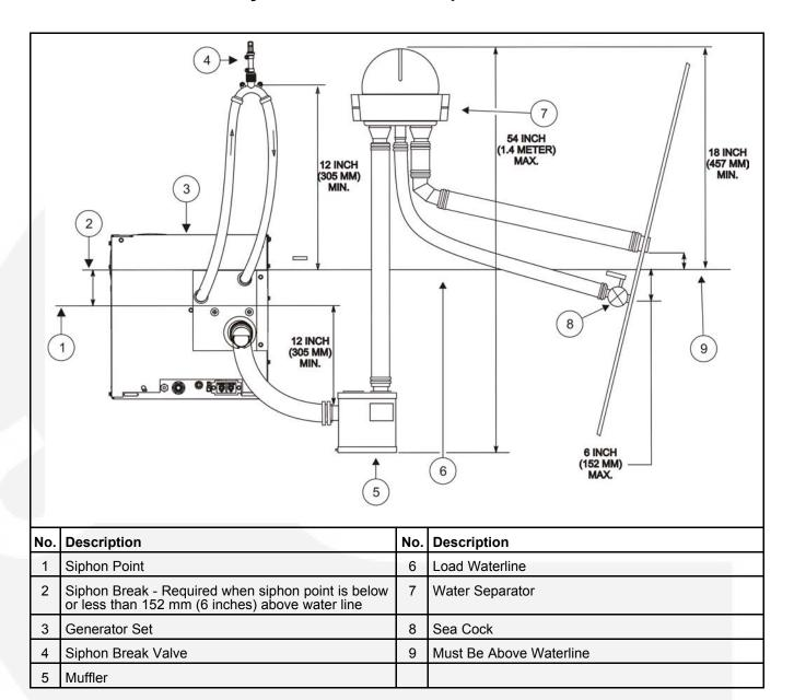
FIGURE 6. TYPICAL WET EXHAUST SYSTEM WITH WATER SEPARATOR
