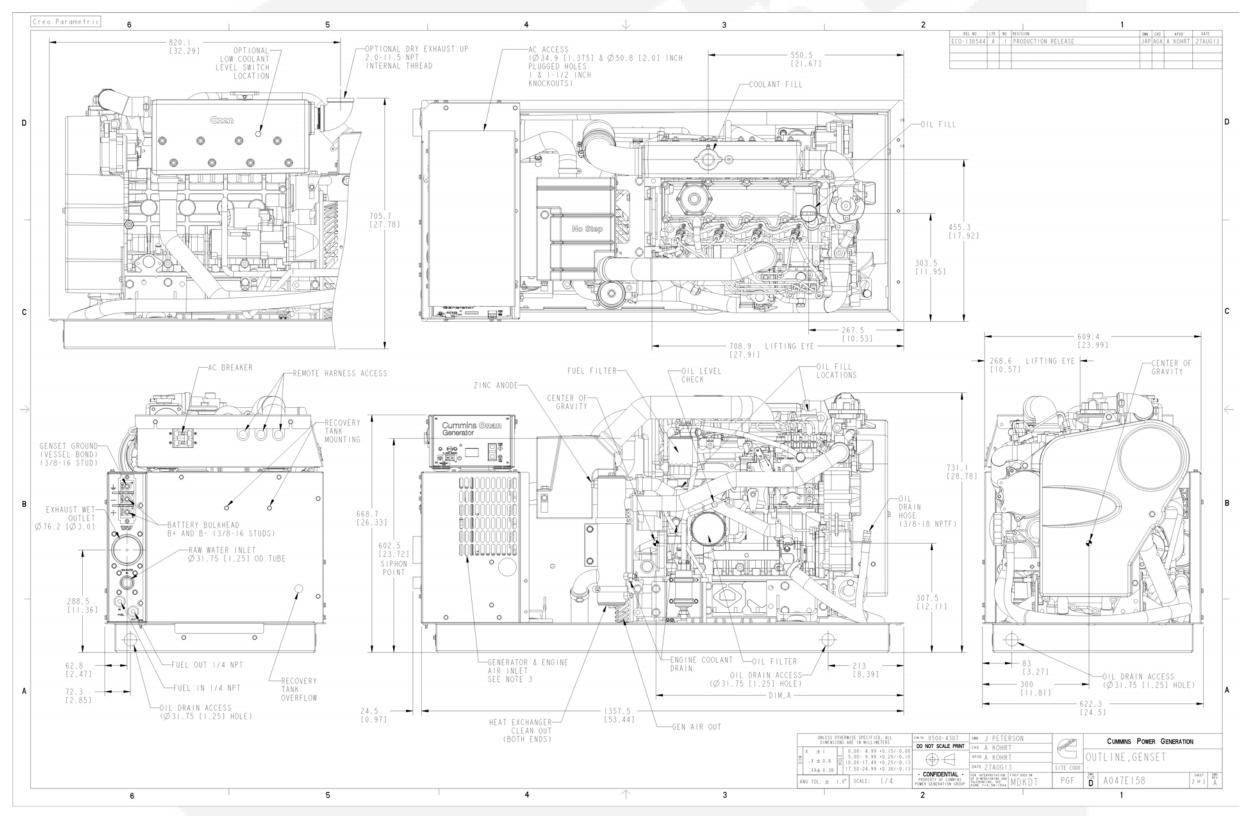
FIGURE 22. MDKDS, MDKDT, MDKDU OUTLINE DRAWING (SHEET 2)
