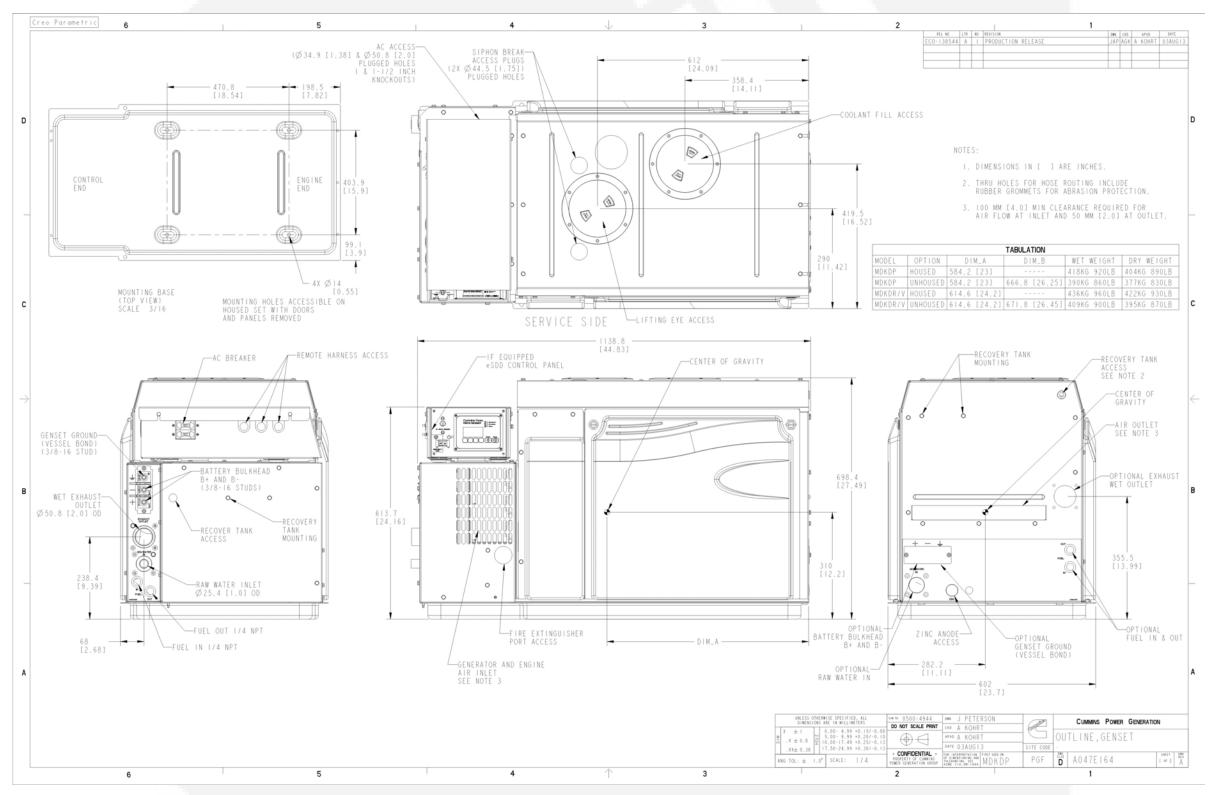
FIGURE 18. MDKDP, MDKDR, MDKDV OUTLINE DRAWING (SHEET 1)
