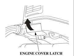
1. Unlock and remove the engine cover (p. 64).
