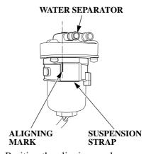
11. Position the aligning mark as shown in the figure when installing the suspension strap on the water separator.
