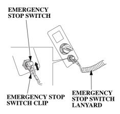
1. Put the emergency stop switch clip in the emergency stop switch, and attach the emergency stop switch lanyard securely to the operator or to the operator's PFD (Personal Flotation Device). The engine will not start or run unless the emergency stop switch clip is in the emergency stop switch.
