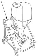
If the outboard motor will be removed from the boat for storage, we recommend storing it vertically by mounting it on a commercially available stand.
