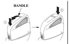
3. While pulling the handle on the engine cover toward you, push the front end of the engine cover down until you hear a click (1), and then push the rear end down until you hear a click (2).
