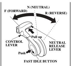
The fast idle button allows you to increase the idle speed without engaging the drive gears. Move the control lever forward or reverse after pushing in the fast idle button to increase the idle speed. It is necessary to position the control lever in the N (neutral) position to push in the fast idle button.
