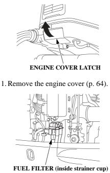
2. Looking through the translucent strainer cup, check the fuel filter for water accumulation or sediment. If the fuel filter is clogged, refer to fuel filter replacement procedure (p. 78) to remove the filter and clean it.
