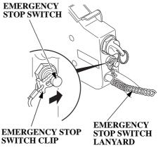
1. Put the emergency stop switch clip in the emergency stop switch, and attach the emergency stop switch lanyard securely to the operator or to the operator's PFD (Personal
