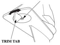
Adjust the trim tab with the engine stopped. Loosen the bolt above the trim tab, turn the trim tab, and then tighten the bolt securely.
