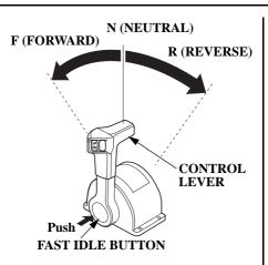
The fast idle button allows you to increase the idle speed without engaging the drive gears. Move the control lever forward or reverse after pushing in the fast idle button to increase the idle speed. It is necessary to position the control lever in the N (neutral) position to push in the fast idle button.
