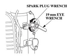
6. Remove the spark plugs with a spark plug wrench and 19 mm eye wrench.
