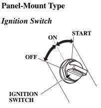
The ignition switch controls the ignition system and the starter motor.
