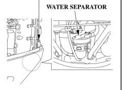
The water separator is located under No. 6 cylinder ignition coil. Water accumulation in the water separator can cause loss of power or hard starting. Check the water separator periodically. Clean it or consult with an authorized Honda Marine dealer for cleaning.
