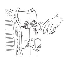
5. Put a teaspoon of engine oil into each spark plug hole to lubricate the inside of the cylinders. Reinstall the spark plugs.
