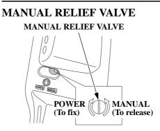
The outboard motor can be tilted manually after opening the manual relief valve. This feature enables the outboard motor to be tilted up or down when no battery is connected.
