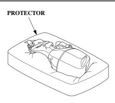
If it is necessary to store the outboard motor horizontally, drain the vapor separator (p. 89 - 90), and drain the engine oil (p. 67), before removing the outboard motor from the boat.
