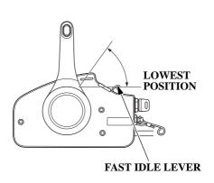
3. Leave the fast idle lever in the OFF (fully lowered) position.
