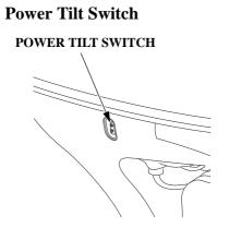
The power tilt switch is located on the engine pan. It is a rocker switch with UP and DN (down) positions for changing the angle of the outboard motor.
