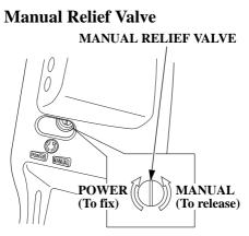
The outboard motor can be tilted manually after opening the manual relief valve. This allows the outboard motor to be tilted up or down when no battery is connected.
