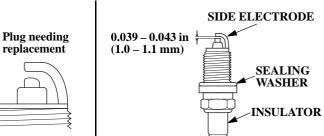
7. Inspect the spark plugs. Replace them if the electrodes are worn, or if the insulators are cracked or chipped. 8. Measure the spark plug electrode gap with a wire-type feeler gauge. Correct the gap, if necessary, by carefully bending the side electrode.
