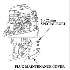
3. Remove the  $6 \times 22$  mm special bolt and remove the plug maintenance cover.
