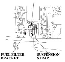
1. Remove the strainer assembly. If it is difficult to remove the strainer assembly by yourself, consult an authorized Honda Marine dealer. Remove the suspension strap from the fuel filter bracket, and then remove the strap from the fuel filter assembly.
