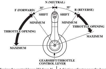
Moving the control lever 35° from N (neutral) selects the gear, and further movement increases engine speed.
