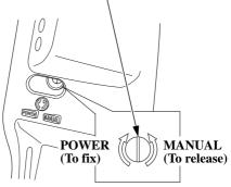
The outboard motor can also be tilted manually after opening the manual relief valve. This feature enables the outboard motor to be tilted up or down when no battery is connected. For manual tilting, use a screwdriver to turn the valve counterclockwise 1 or 2 turns. Close the valve firmly after positioning the engine.
