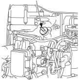
4. If the oil level is low, remove the oil filler cap, and add oil to reach the upper limit mark shown on the dipstick. Use the oil recommended on p. 69.
