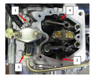
Figure 9: Cylinder head bolts
