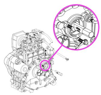
Figure 10: Turning tool to move to Top Dead Center position
