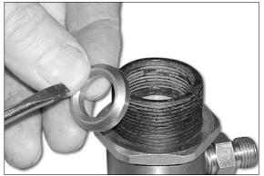
Fit the new gasket kit according to the component sequence shown in the figure.
