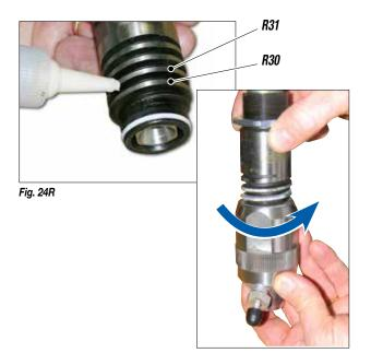
Use a 36 mm spanner to screw on the pump unit (R9).
