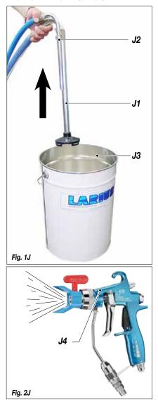
Plunge the suction (J1) and the recirculation hoses (J2) in the thinner container (J3). Set pressure to the mimimum and by keeping the nozzle below the thinner level in the container, spray until the thinner has been recycled during three or five minutes.
