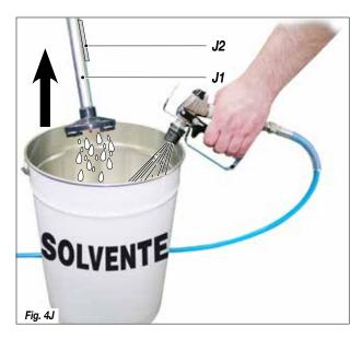
After washing, in case a long period of downtime is foreseen or if a water-based product has been used, it is advisable to lubricate the inner parts (pumping group), by sucking the hydraulic oil with the pump, without discharging it.
