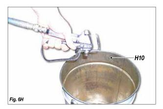
Never operate the pump without the product, in order to prevent the gaskets to be damaged.
