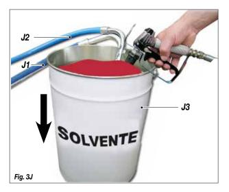
• By going on spraying, lift the suction (**J1**) and the recirculation hoses (**J2**), in order to drain out all the thinner. Then stop the pump, by closing the air tap.
