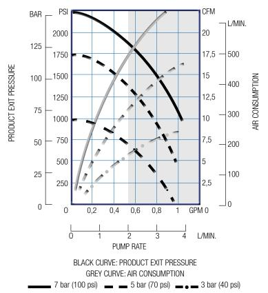
The pump can operate in continuous mode when the rate is limited to the white area. Outside this area, the speed shall be intermittent.
