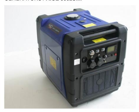
The petrol AIGE 3002SMP inverter unit is equipped with a multi-phase alternator+ inverter board with stabilised 220V single-phase output. The THD (total harmonic distortion) value is less than 2%, the voltage accuracy is between +1% and -1%.
