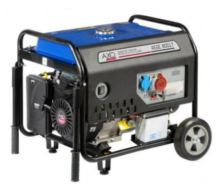
The semi-silent petrol AEGE 8001T generator is equipped with a three-phase alternator with neutral available, THD (total harmonic distortion) value less than 6% and voltage accuracy between +1.5% and -1.5%.
