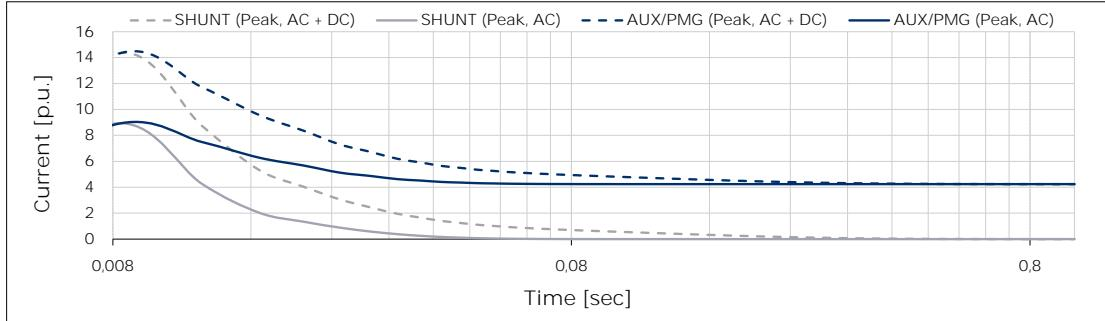
Above curves are based on a three-phase short circuit
