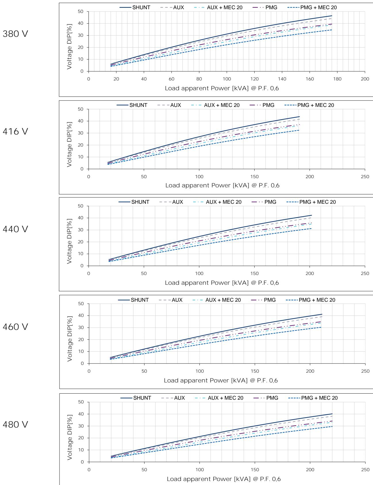
For P.F. different from 0,6 the following simplified formula can be used:  $\Delta V (@ P.F.) = \Delta V (@ 0,6) * \sin(\arccos(P.F.)) / 0,8$
