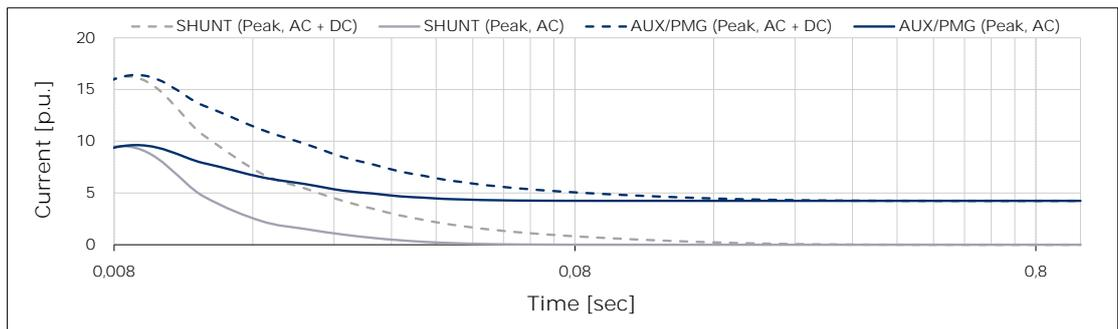
Above curves are based on a three-phase short circuit
