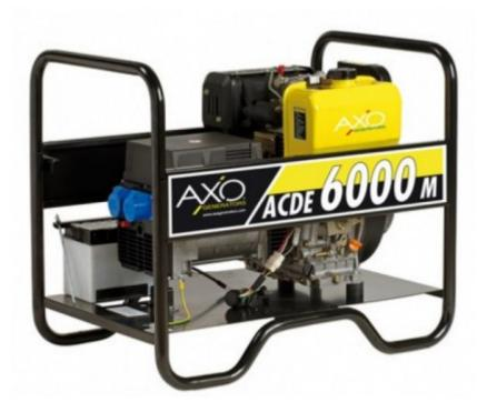
The ACDE 6000M generator for worksites is equipped with a diesel engine, single-phase alternator designed and manufactured in Italy. The THD (total harmonic distortion) value is less than 6% and the voltage accuracy is between +5% and -10%.
