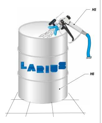
• Lift again the suction pipe and remove the solvent tank.
