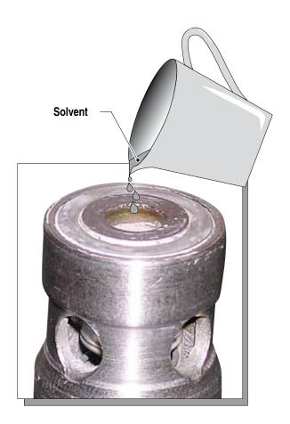
If the quantity of solvent a few minutes later is still identical to that added previously, the ball's seal in its seating is ensured;
