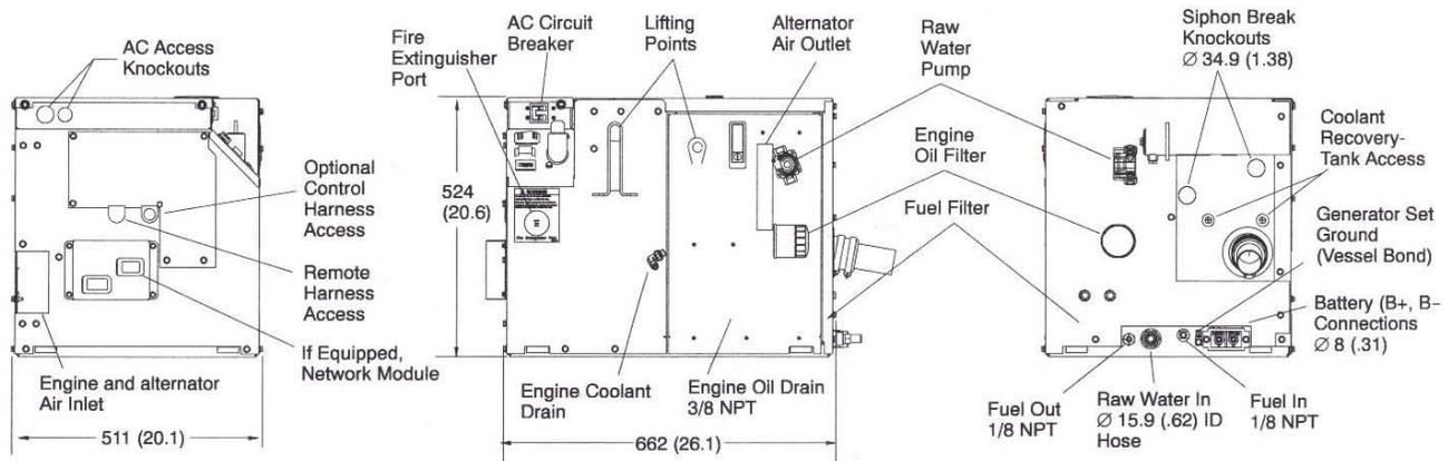
**Note:** This outline drawing is provided for general reference only and is not intended for design or installation. For more information see Operation and Installation manuals or obtain drawing 500-4718 and wiring diagram from your distributor/dealer.
