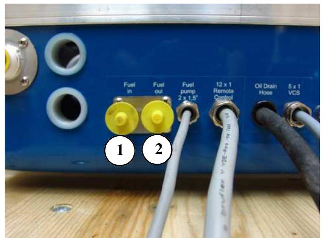
Fig. A.3.4-2: Fuel connections
