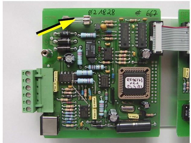
Fig. E.3.2-1: Fuse on VCS board
