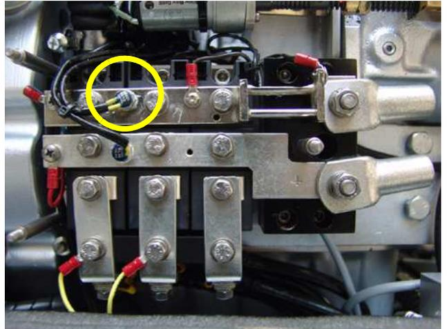
Fig. A.3.7-5: Thermo-switch on the (-)-connection bar
