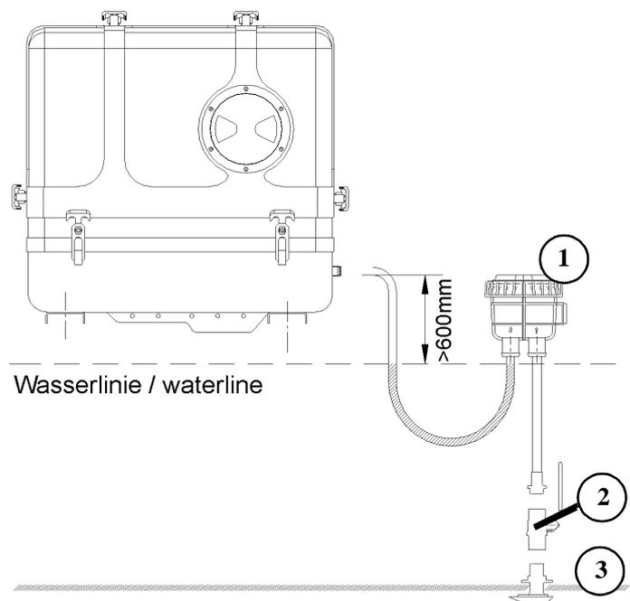
Fig. C.5.0-1: Raw water filter
