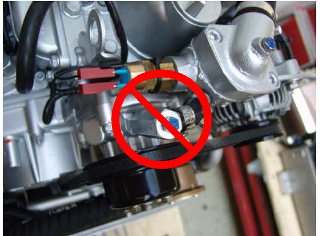
Fig. D.6-5: entilation screw - water pump
