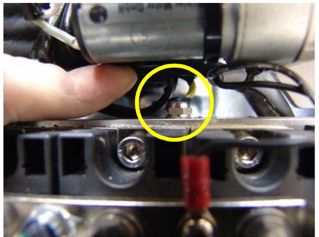
Fig. A.3.7-7: Thermo-switch on the rectifier block
