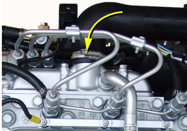
Fig. A.3.5-4: Induction elbow
