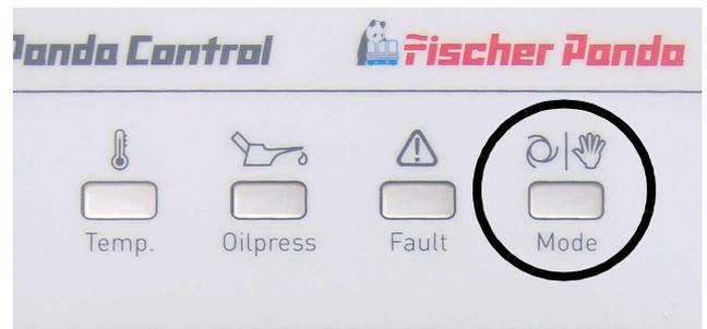
Errors will be collected and displayed only when the generator is running. The first encountering errors displayed in the panel. All other errors will be collectet and can be seen under the menu point „Errors“.
