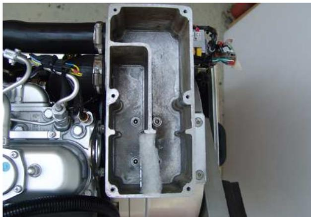
Fig. D.5-2: Air suction housing
