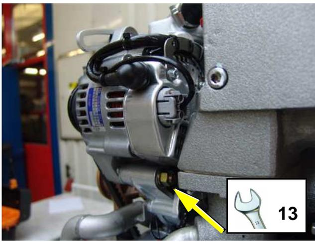
Fig. D.7-3: Fixing screw - DC-alternator
