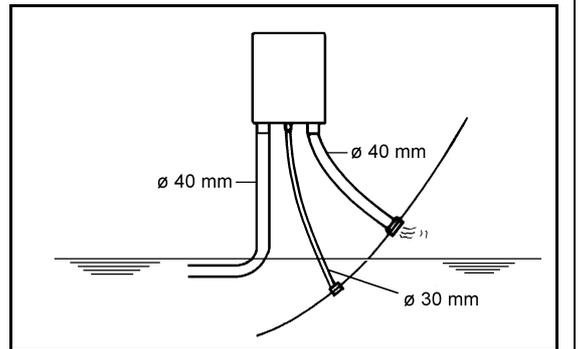
Fig. B.5.2-1: Exhaust/water separator
