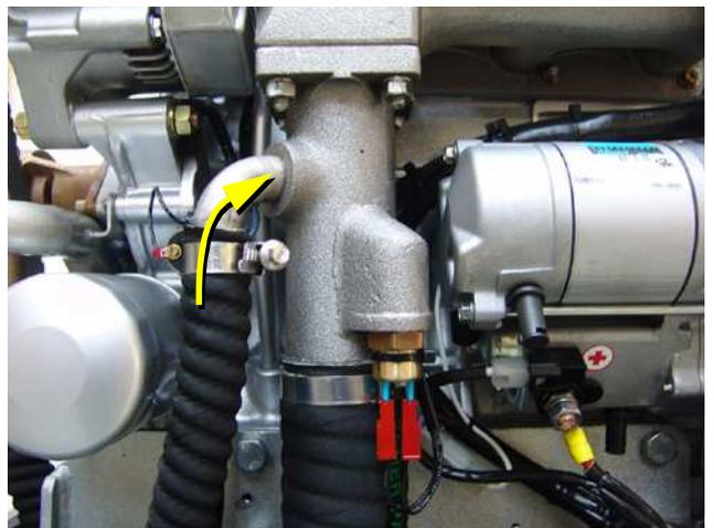
Fig. A.3.2-8: Cooling water injector port
