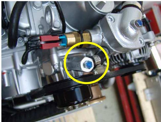
Fig. A.3.3-8: Ventilation screw cooling water pump
