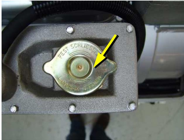
Fig. A.3.3-1: Cooling water filler neck
