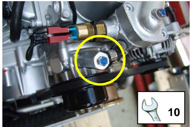
Fig. D.6-2: Ventilation screw - water pump
