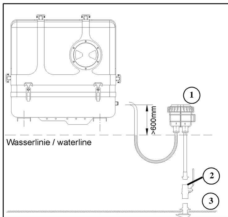
Fig. B.3.4-1: Raw water filter
