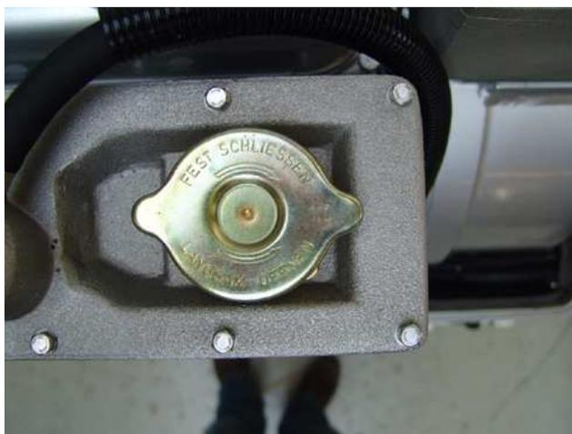
Fig. B.4.2-1: Cooling water filler neck
