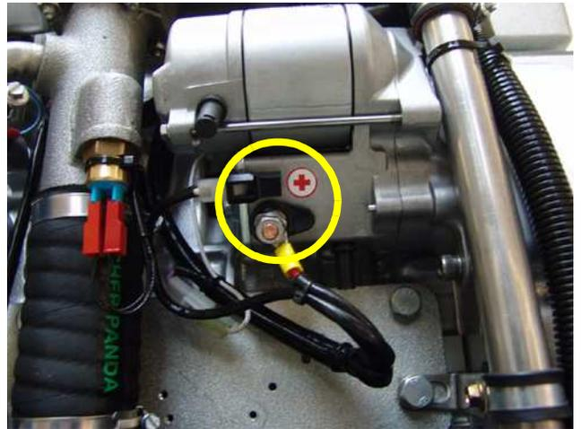
Fig. B.7.1-1: Connection positive battery cable
