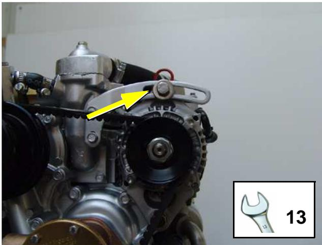
Fig. D.7-1: Fixing screw - DC-alternator
