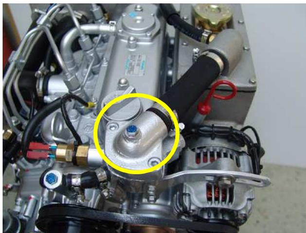
Fig. A.3.3-9: Ventilation screw thermostat housing
