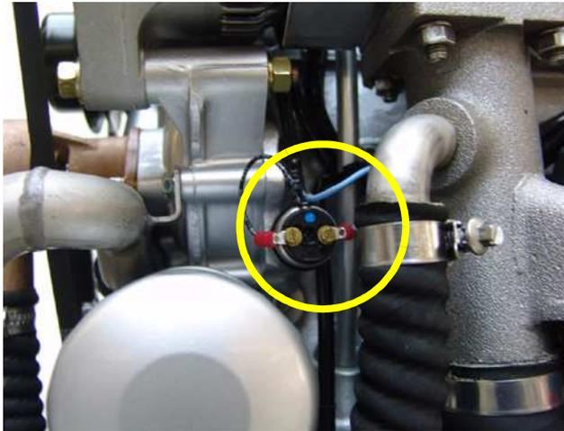
Fig. A.3.7-8: Oil pressure switch
