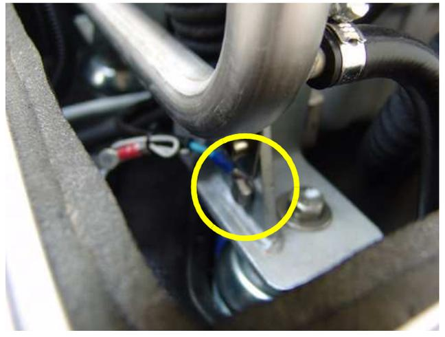
Fig. B.7.1-2: Connection negative battery cable
