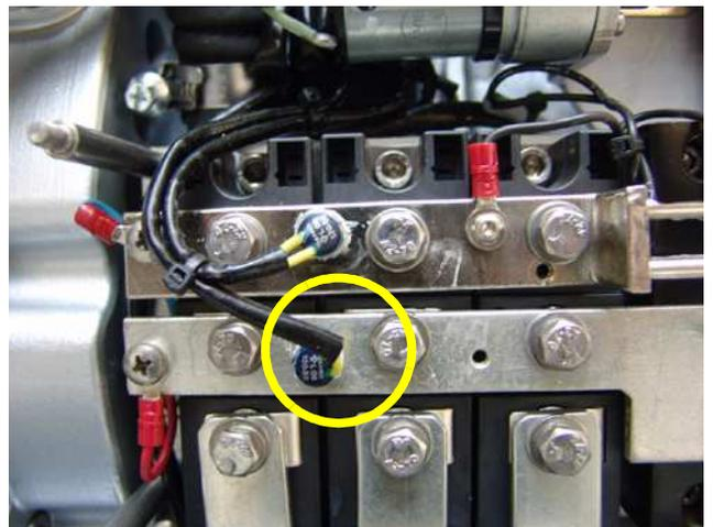
Fig. C.1-6: Thermo-switch on the (+)-connection bar
