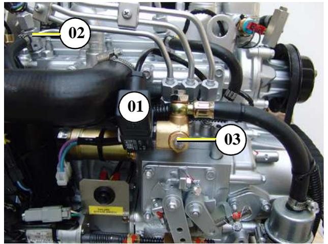
Fig. E.5.2-1: Fuel solenoid valve
