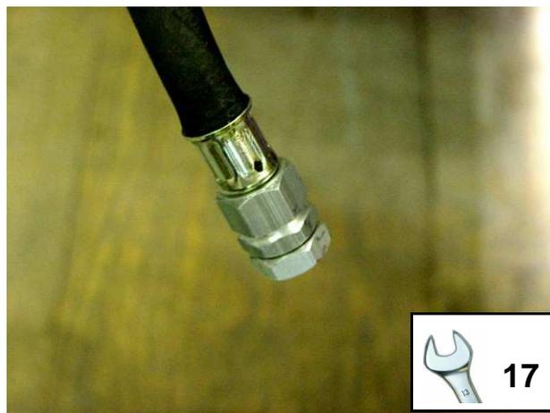
Fig. D.3-2: Oil drain screw
