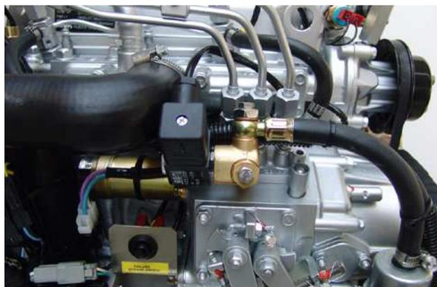
Fig. B.6.5-1: Fuel solenoid valve
