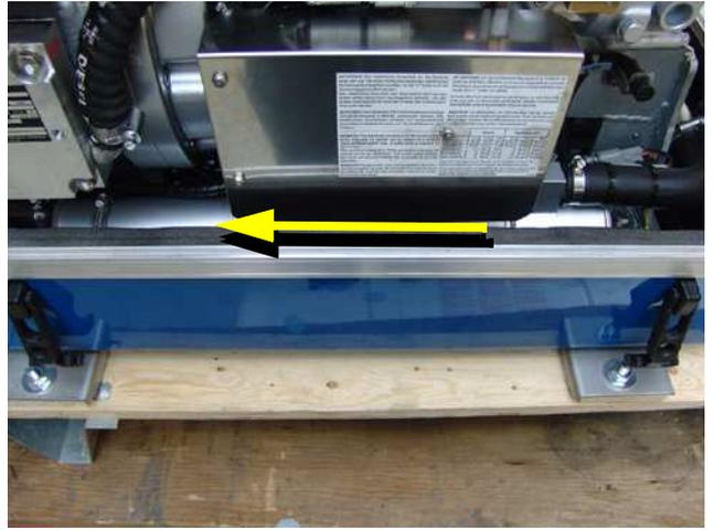
Fig. A.3.2-6: Heat exchanger
