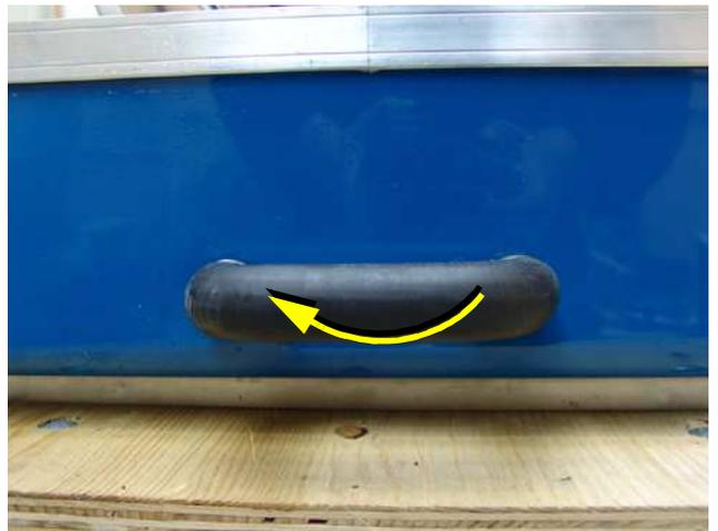
Fig. A.3.2-7: Connection ventilation valve
