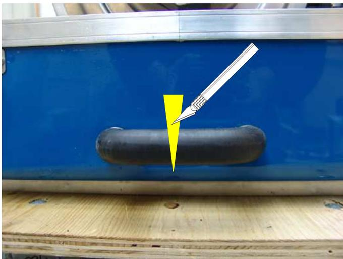
Cut the hose rubber for the external valve vent.....
