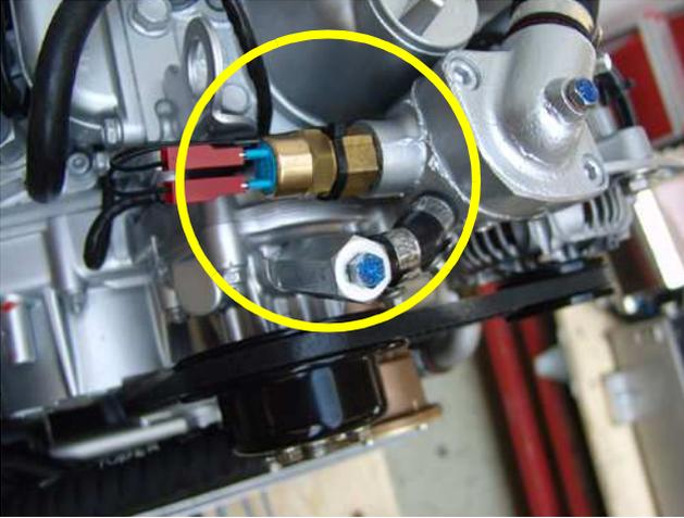
**Thermo-switch at thermostat housing**
