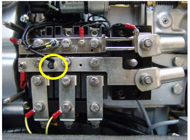
Fig. A.3.7-6: Thermo-switch on the (+)-connection bar
