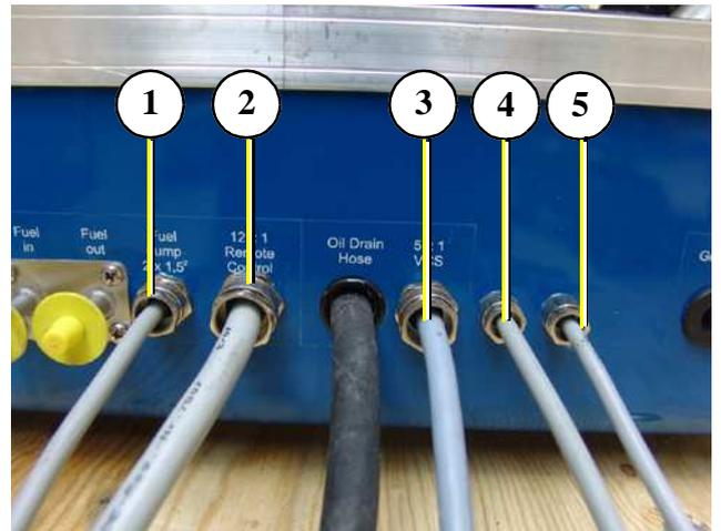
Fig. A.3.6-3: Electrical connections
