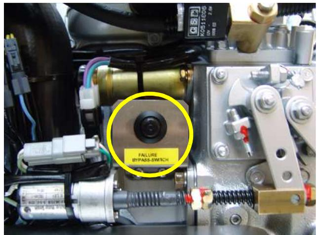
Fig. A.4.5-1: Failure bypass switch
