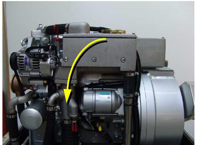
Fig. A.3.5-6: Water-cooled exhaust elbow
