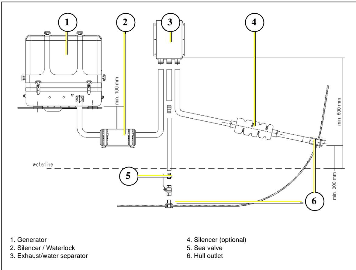
Fig. B.5.3-1: Installation exhaust/water separator - example
