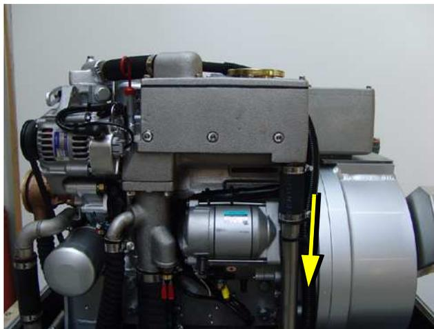
Fig. A.3.3-3: Ventilation pipe
