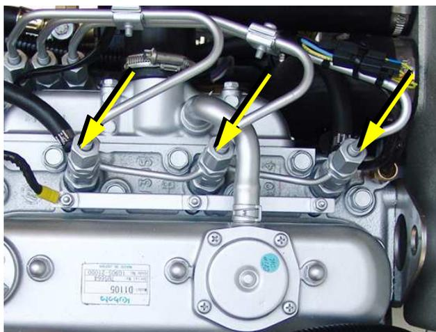
Fig. A.3.4-5: Injection nozzle
