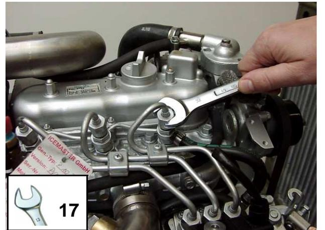
Fig. D.4-3: Injection nozzle
