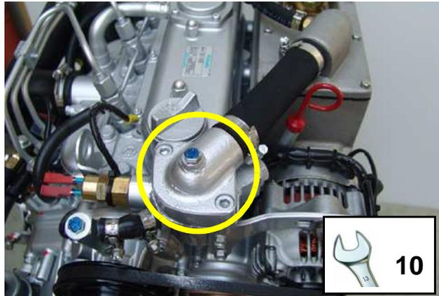
Fig. D.6-3: Ventilation screw - thermostat housing
