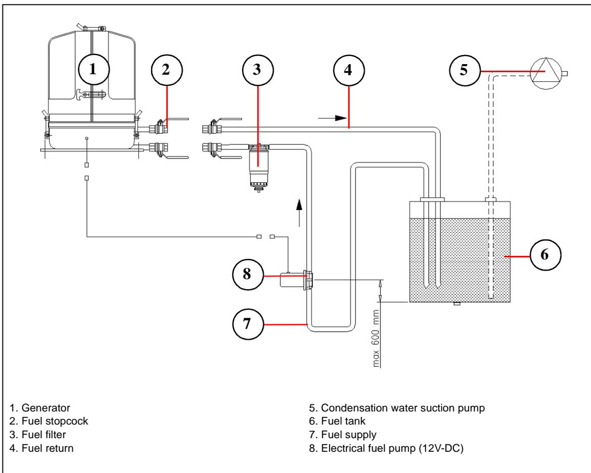
Fig. B.6.1-1: Installation fuel system - example
