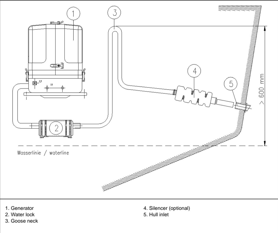
Fig. B.5.1-1: Installation stanrd exhaust system - example
