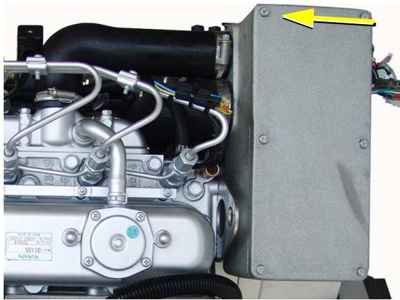
Fig. D.5-1: Air suction housing
