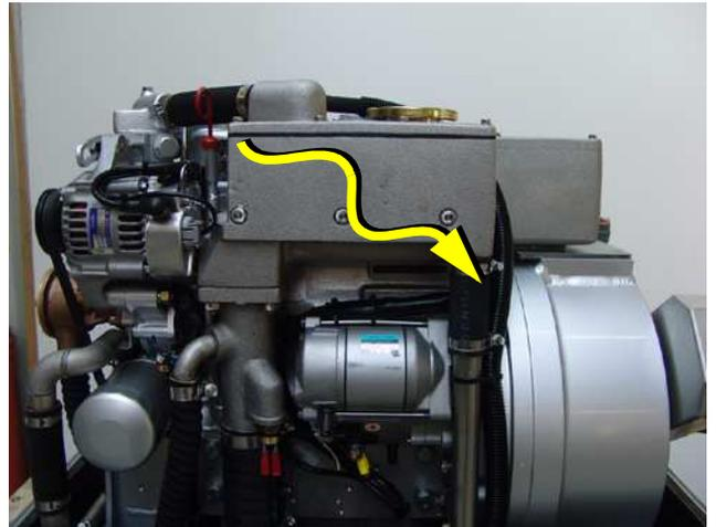
Fig. A.3.3-10: Water-cooled exhaust elbow
