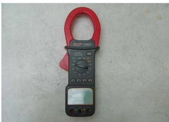
Current clamp (DC for synchron generators; AC for asynchron generators)
