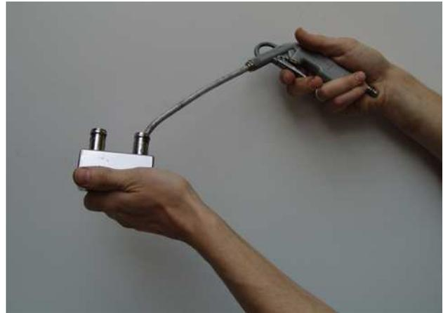
Fig. H.3-9: Cleaning with air
