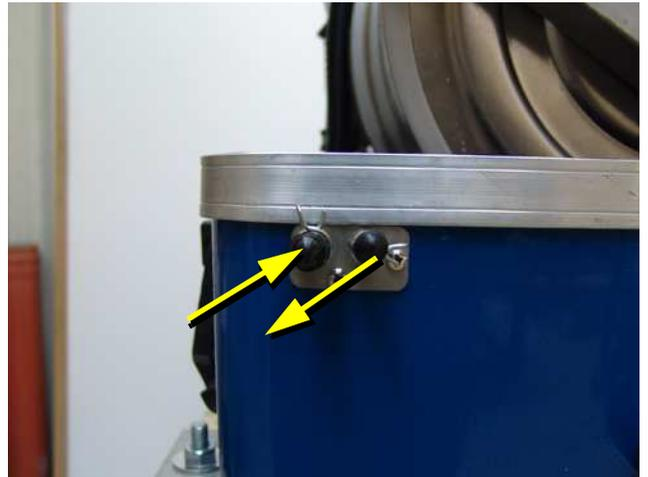
Fig. A.3.3-4: External expansion tank
