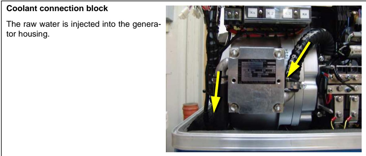
Fig. A.3.2-5: Coolant connection block
