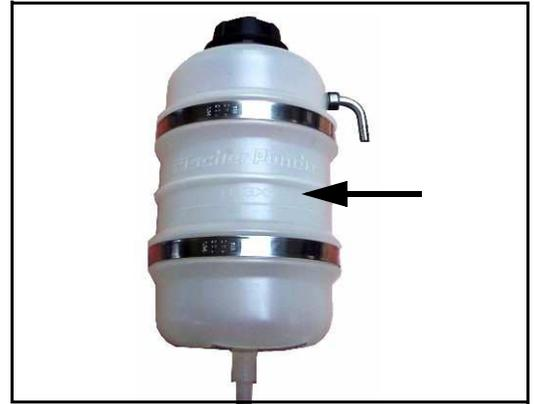
Fig. B.4.2-5: External cooling water expansion tank
