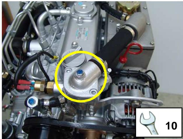
Fig. B.4.2-2: Ventilation screw -thermostat housing
