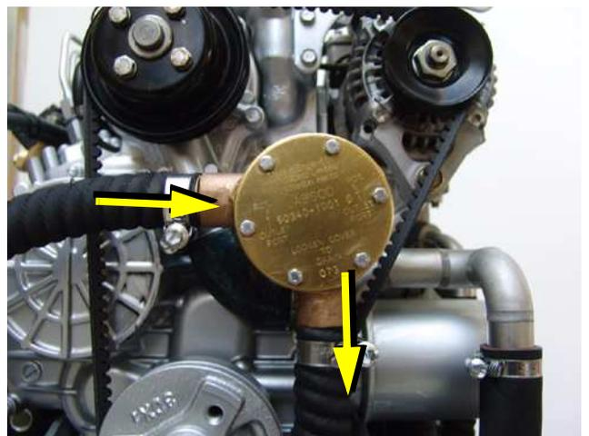
Fig. A.3.2-2: Raw water impeller pump
