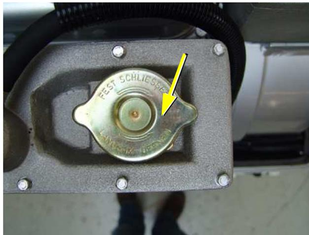
Fig. D.6-4: Cooling water filler neck
