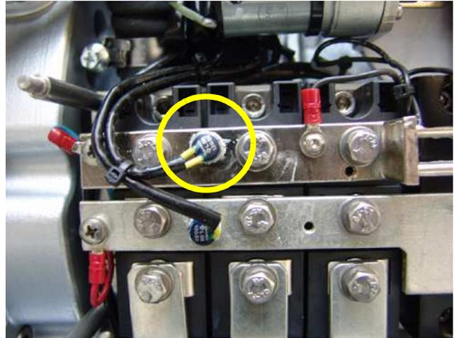
Fig. C.1-5: Thermo-switch on the (-)-connection bar
