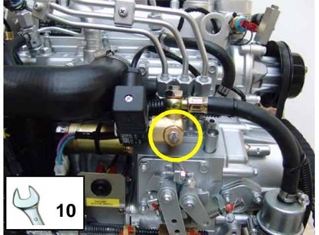
Fig. D.4-2: Ventilation screw - fuel solenoid valve
