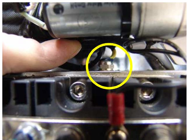
Fig. C.1-7: Thermo-switch on the rectifier block
