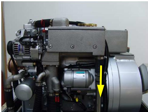
Fig. A.3.3-2: Freshwater backflow
