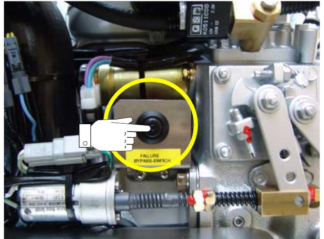
Fig. C.1.3-1: Failure bypass switch
