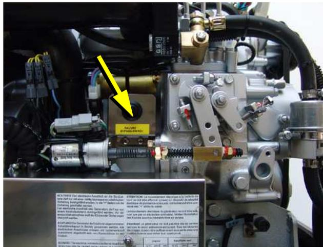
Fig. E.5.3-1: Failure bypass switch
