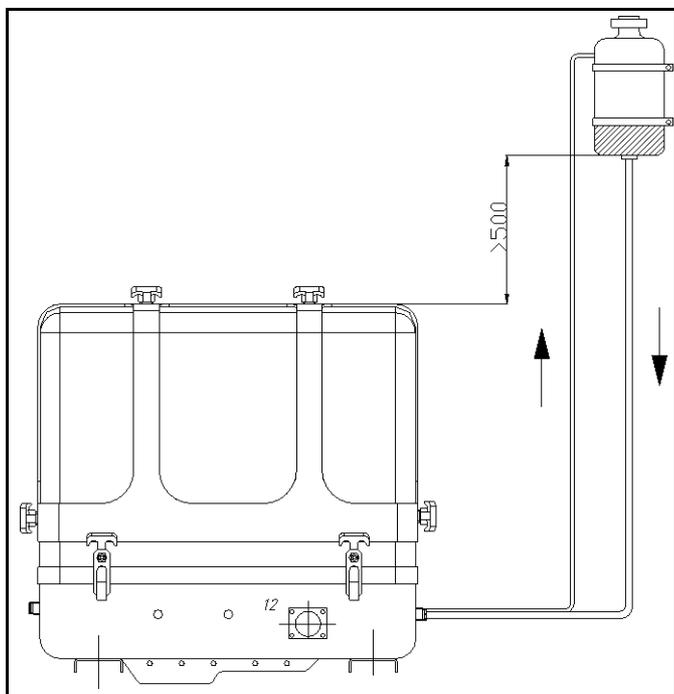
Fig. B.4.1-1: External cooling water expansion tank
