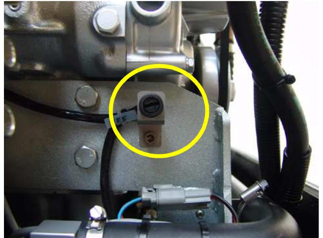
Fig. A.3.6-9: Fuse for voltage sense
