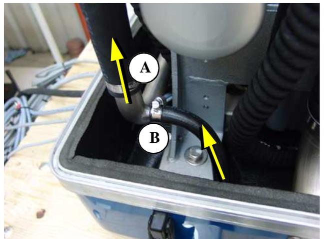
Fig. A.3.3-6: Cooling water injection
