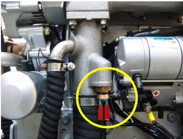
Fig. A.3.7-3: Thermo-switch at exhaust connection
