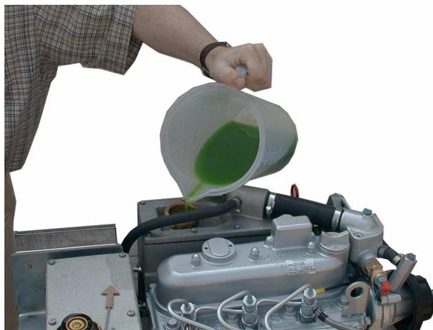
Fig. B.4.2-4: Cooling water filler neck
