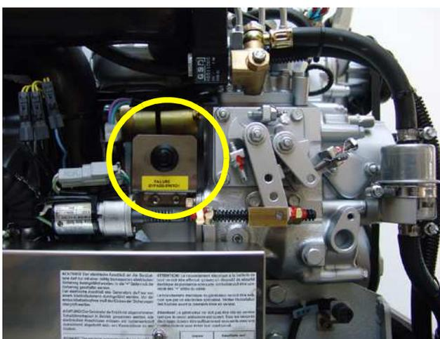
Fig. A.3.7-9: Failure bypass switch
