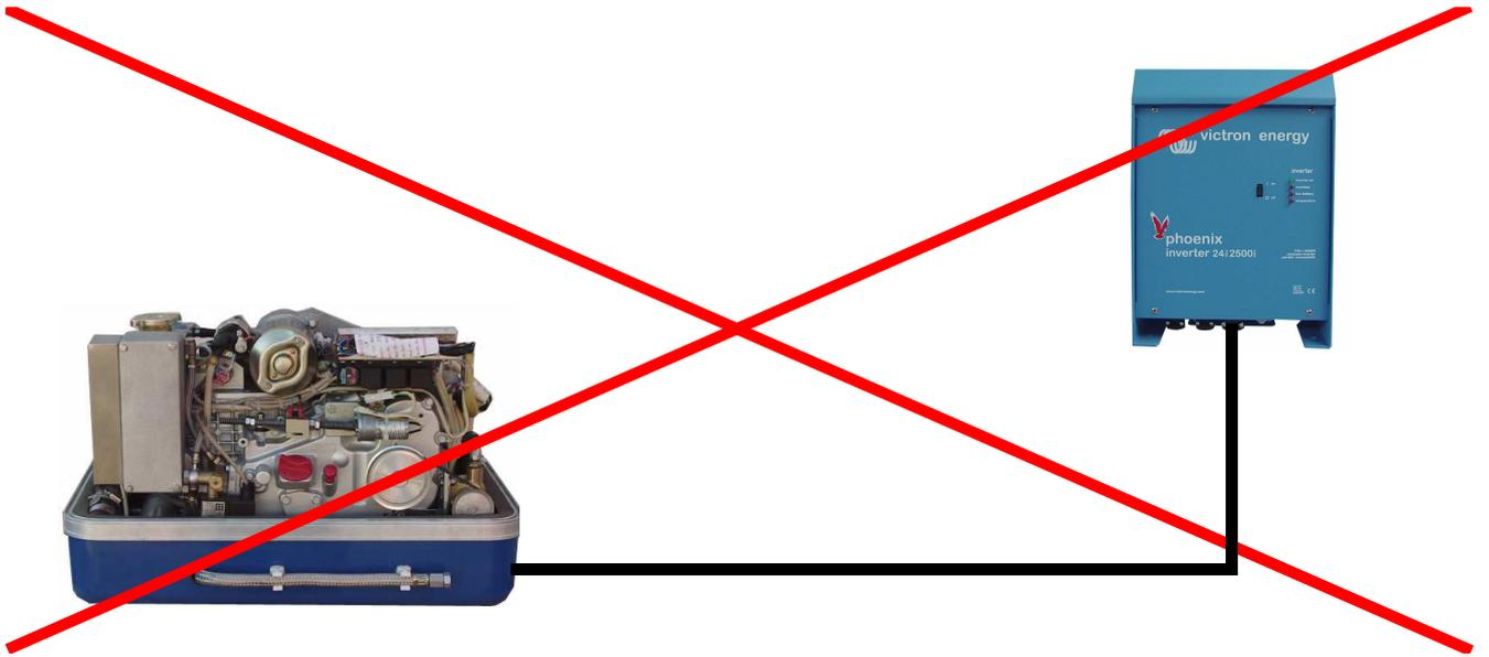
**The Inverter generates voltage peaks, which can destroy the rectifier rectifiers of the generator!**
