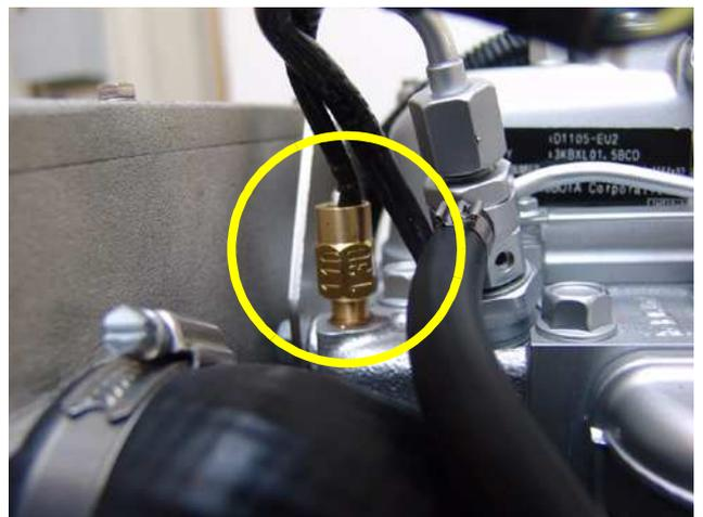
Fig. A.3.7-1: Thermo-switch at cylinder head
