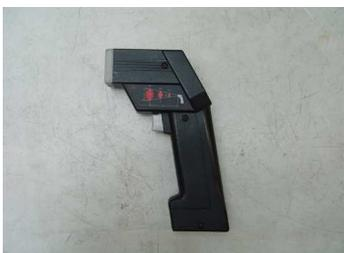
Infrared temperature measuring pistol
