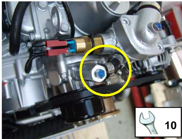
Fig. B.4.2-3: Ventilation screw - water pump
