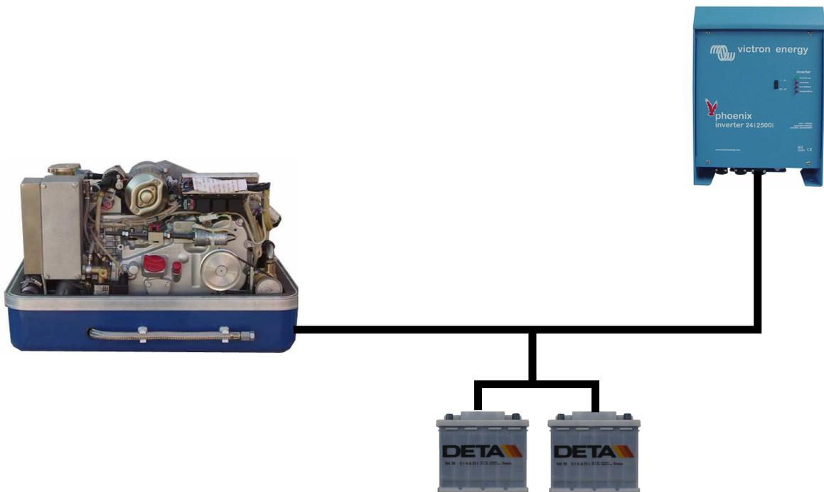
**A battery must always be connected to the inverter as a capacity!**
