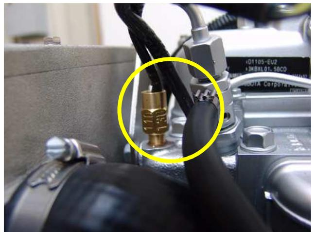
Fig. C.1-1: Thermo-switch at cylinder head
