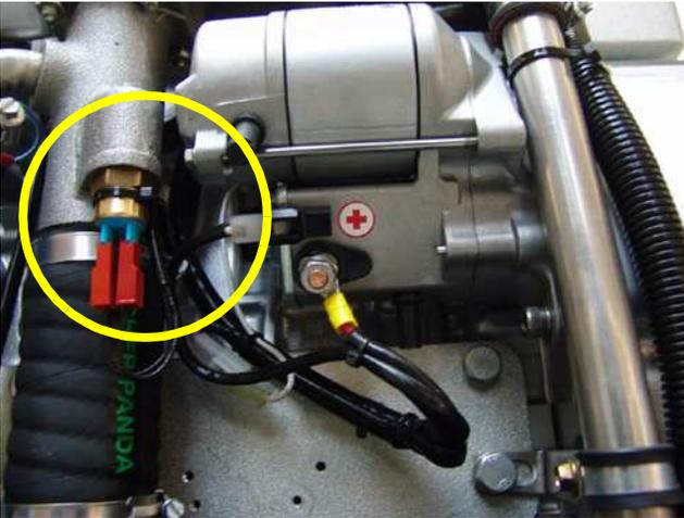
**Thermo-switch at exhaust connection**
