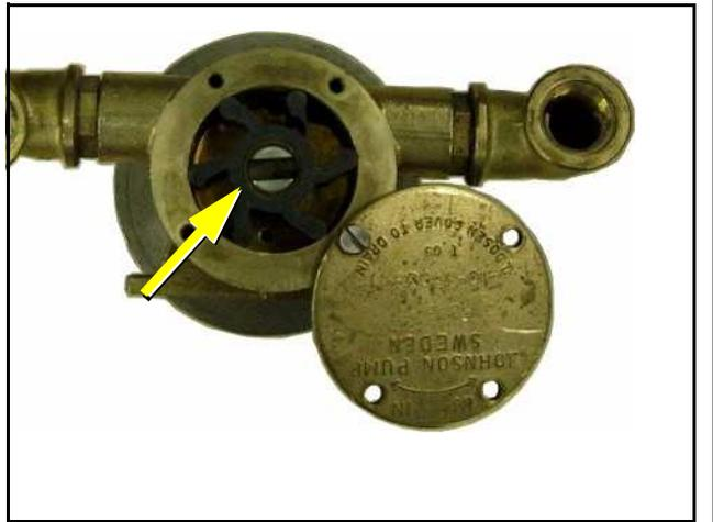
Fig. D.8.3-3: Impeller
