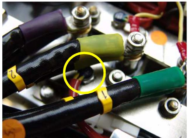
Fig. A.3.6-6: Thermo-switch on the (+)-bar
