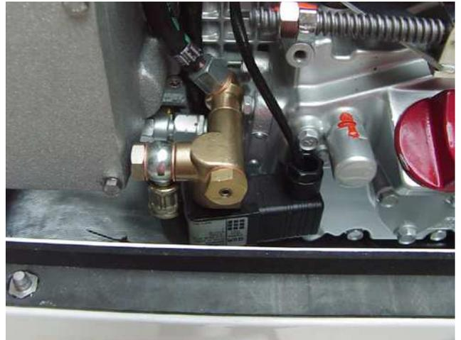
Fig. E.2.2-1: Fuel solenoid valve
