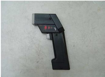
Infrared temperature measuring pistol
