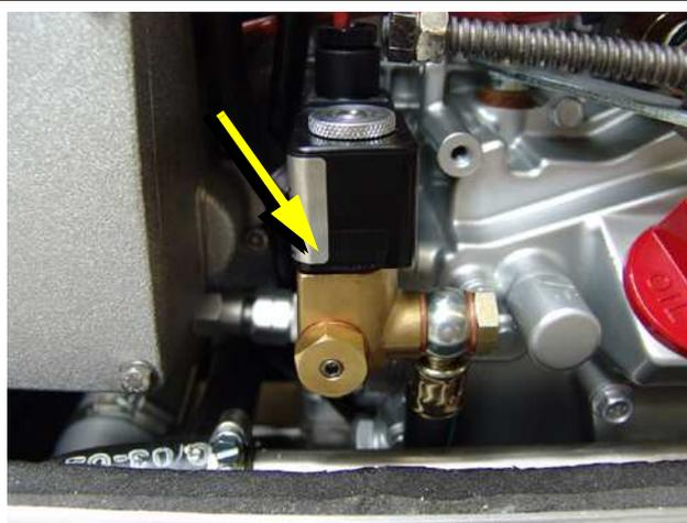
Fig. A.3.3-3: Fuel solenoid valve
