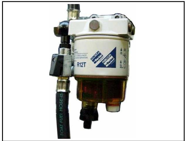
Fig. D.3.1-1: External fuel filter
