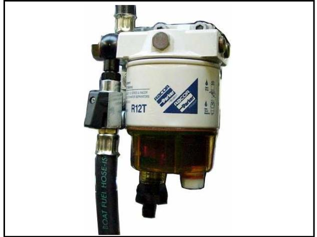
Fig. C.6.4-1: External fuel filter
