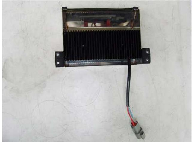
Fig. A.3.5-10: DC&DC/converter
