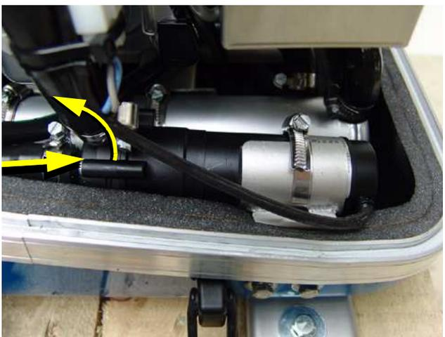
Fig. A.3.2-4: Internal cooling water pump
