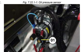
2. Loosen and remove oil pressure sensor 6R3 using a wrench with W.A.F. of 17 mm. A large piece of cloth or absorbent tissue must be placed under the connection to prevent escaping oil from running into the capsule.
