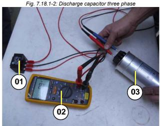
Fig. 7.18.1-3: Capacitor checking
