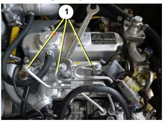
Fig. 7.26-4: Injection nozzles
