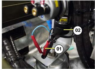
Fig. 7.22-2: Oil pressure sensor
