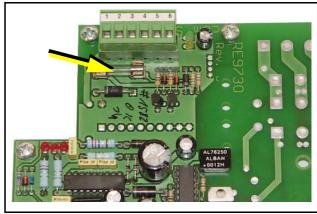
Fig. 8.7.4-1: Fuse for the actuator at the remote control panel
