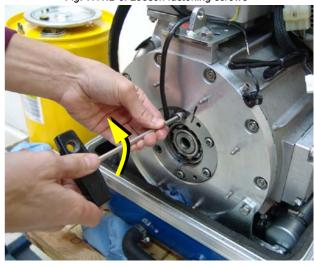
As shown, screw in 3 lifting screws M8x50 as far as possible by hand.
