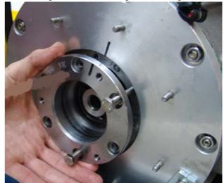
Carefully press the bearing case with a soft-head hammer (or a hammer plus mandrel) in its hub.
