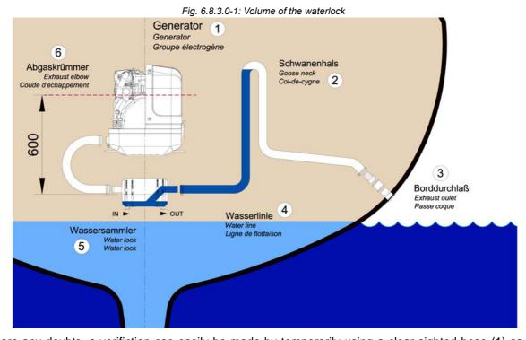
If there are any doubts, a verifiction can easily be made by temporarily using a clear-sighted hose (1) as exhaust hose. In that way, the cooling water level can be checked very easily.
