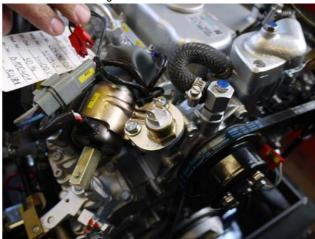
4. Loosen thermoswitch with a wrench with W.A.F. 22 mm.
