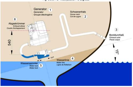
Fig. 6.8.3.1-2: Tilted position 15 degrees
