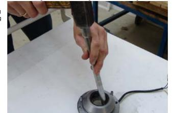
Fig. 7.11.2-8: Knocking out the ball bearing
