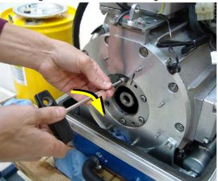
Fig. 7.10.1.3-5: Screw in thread rod
