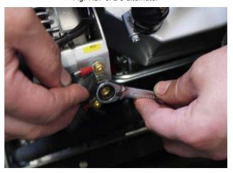
5. Remove nut and washer of the exciter terminal (grey cable) with a wrench with W.A.F. 8 mm.
