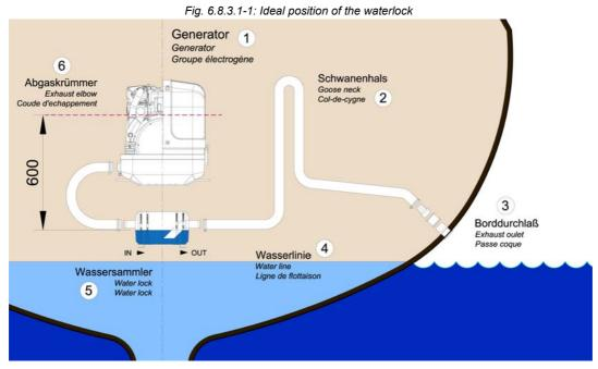
In Fig. 6.8.3.1-1, the waterlock is mounted in center underneath the generator. When the ship tilts, the position of the waterlock related to the critical point at the exhaust hose, changes only slightly.
