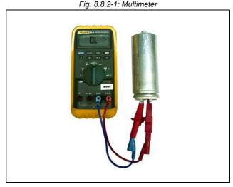
Should a steady sound or no sound be heard, the capacitors are defective and must be replaced.
