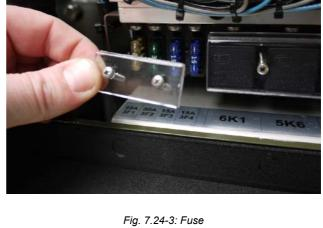
3. Using the fuse extraction tool, remove the fuse and replace it with a new one.
