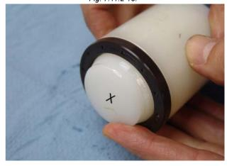
Fig. 7.11.2-17: Fitting the shaft sealing ring
