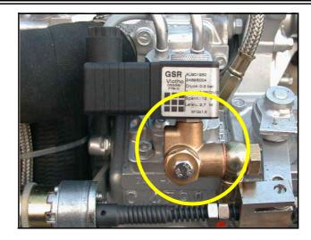
Vent Screw at the fuel stop solenoid valve
