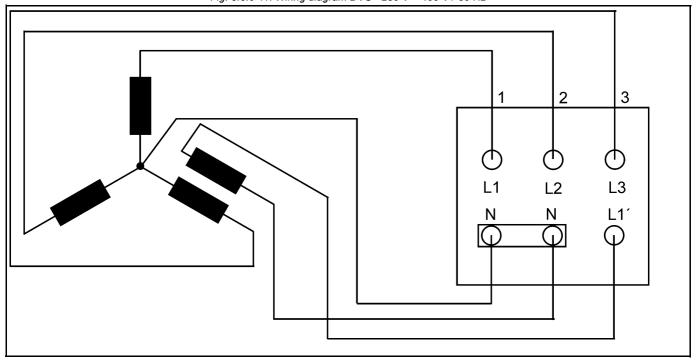
Fig. 8.5.0-11: Wiring diagram DVS - 230 V + 400 V / 50 Hz
