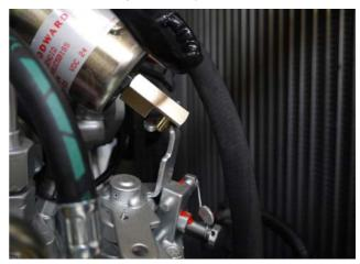
9. Push the throttle to the left and release. Fig. 7.28-8: Stop solenoid
