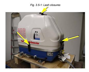
To open the lash closures pull the handle in arrow direction and lift the lash of the closure pin. After lifting of the lashes, the sound isolation cover upper pars can be removed.
