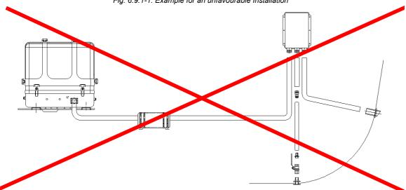
Fig. 6.9.1-1: Example for an unfavourable Installation
