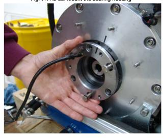
Now carefully press the bearing housing in its seat with a soft headed hammer (or hammer plus mandrel).
