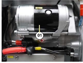
Fig. 7.19-2: Electric starter
