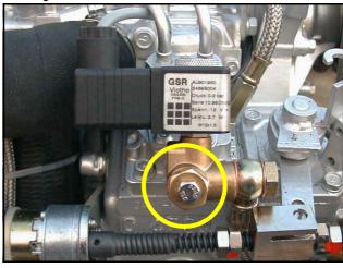
Not all generator models has a fuel solenoid valve. At gener- Note!: ators without fuel solenoid valve, a single ventilation screw is installed.
