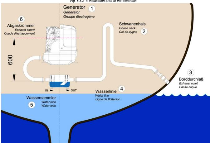
Fig. 6.8.2-1: Installation area of the waterlock
