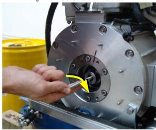
Slide on ball bearing, pressure ladle, grommet up to the shaft, screw on long hexagon nut. Grease/Oil thread rod.
