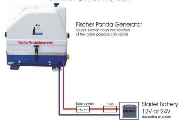
Fig. 1.6-1: Sample diagram for starter battery installation
