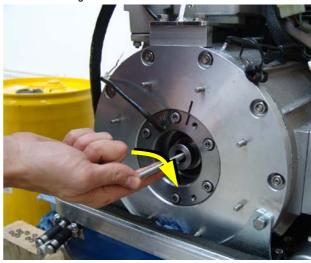
Push the ball bearing, the pressure ladle and the washer up against the shaft, then screw on the hex nuts. Grease/lubricate the thread rod.
