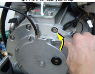
As shown, degrease the spot with a fat solvent and make a mark with a waterproof pen.
