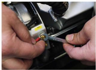
7. Loosen upper fixing screw of the DC alternator with a wrench with W.A.F. 13 mm.
