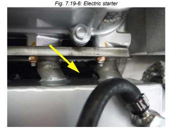
Fig. 7.19-7: Electric starter
