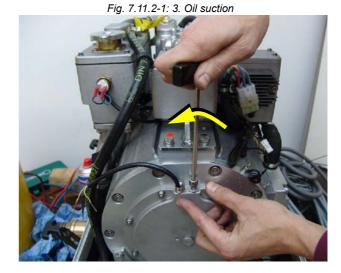
Inserting the hose through the ventilation screws' tap hole.
