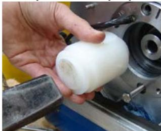
Tighten the fastening screws M8 with 22 to 25 Nm (Tool: Allen wrench SW6).
