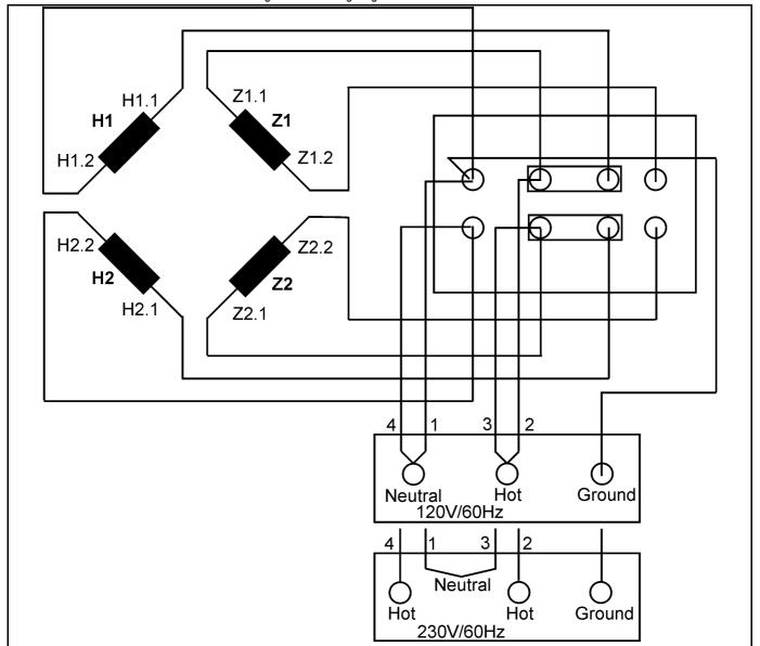
Fig. 8.5.0-6: Wiring diagram HP1 - 120 V / 60 Hz
