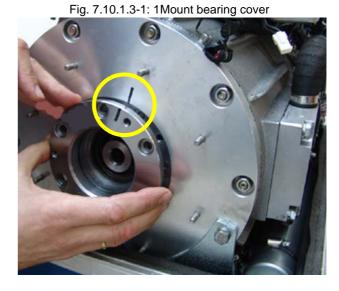
Fig. 7.10.1.3-2: Bearing case mouting
