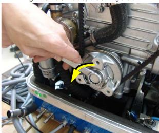
Fig. 7.10.1.3-9: Remove tools and markings
