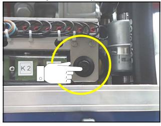
3. Pressing the failure bypass switch for approx 3 - 4 minutes will loosen the ventilation screw located at the fuel solenoid valve. The button must continue to be pressed. whilst opening the screw. A large cloth or Kleenex tissue must be laid beneath the connection to prevent escaping fuel running into the capsule. If the fuel runs out without air bubbles, then the ventilation screw can be closed. Only then may the button be released.
