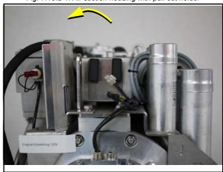
2. Tip the two fasteners 90°
