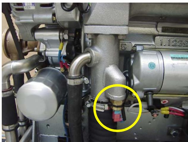
Fig. 4.3.4-3: Thermo-switch at exhaust connection
