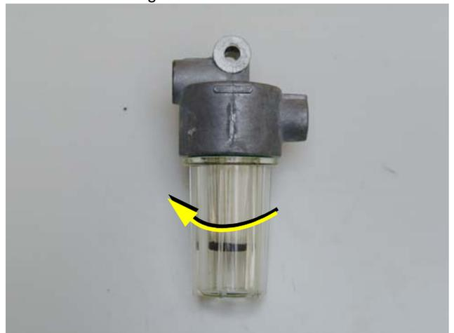
2. Unscrew the filter element from the mount (left hand rotation).
