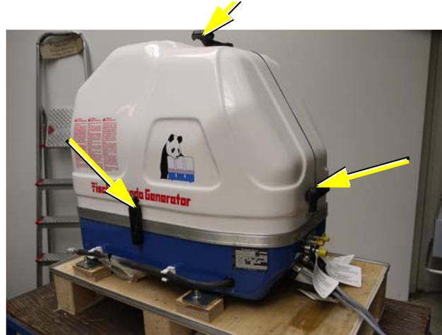
To open the lash closures pull the handle in arrow direction and lift the lash of the closure pin. After lifting of the lashes, the sound isolation cover upper parts can be removed.
