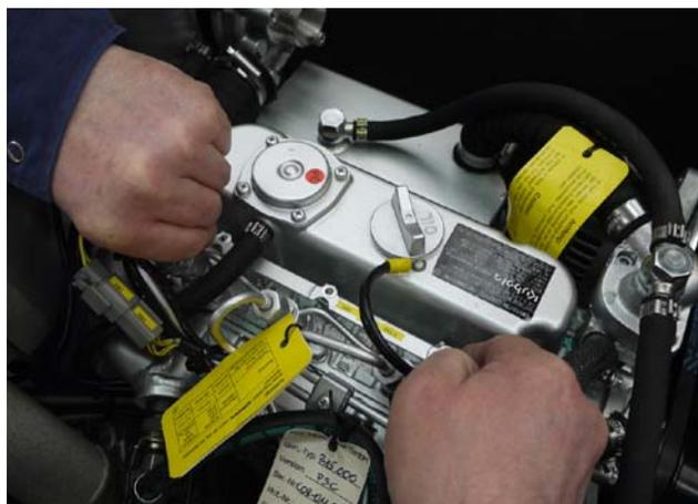
4. Loosen the glow plug using a socket wrench with a long size 10 mm socket.
