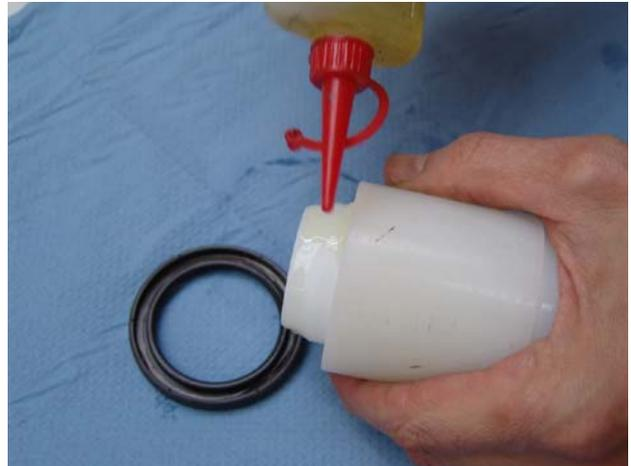
**Push the sealing ring on the mandrel, the open side should point towards the handle. The side marked with „X“ is to be used.**
