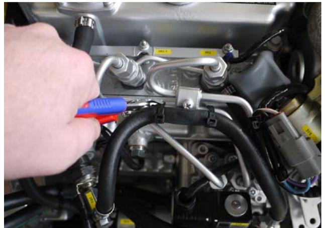
Fig. 7.26-2: Injection nozzles
