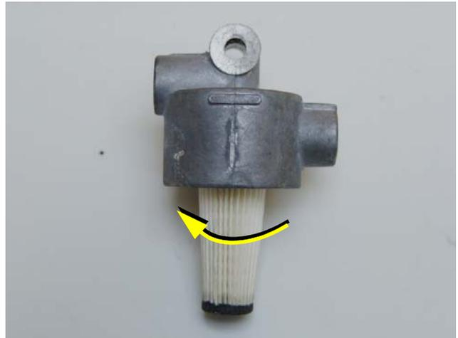
3. Screw the new filter element into the mount.
