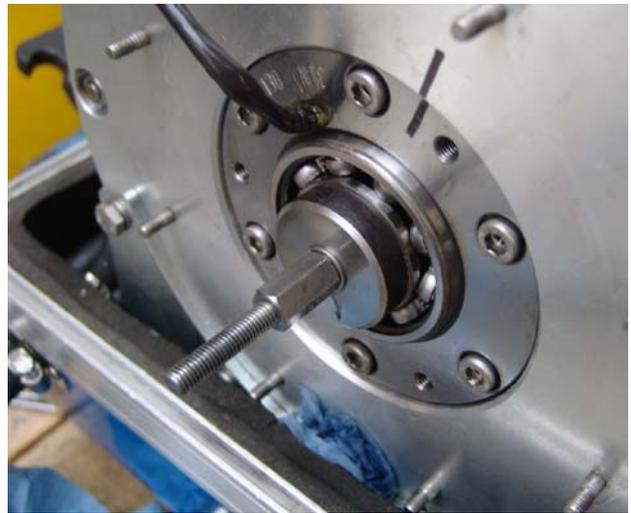
By doing that, the ball bearing is pressed onto the shaft.
