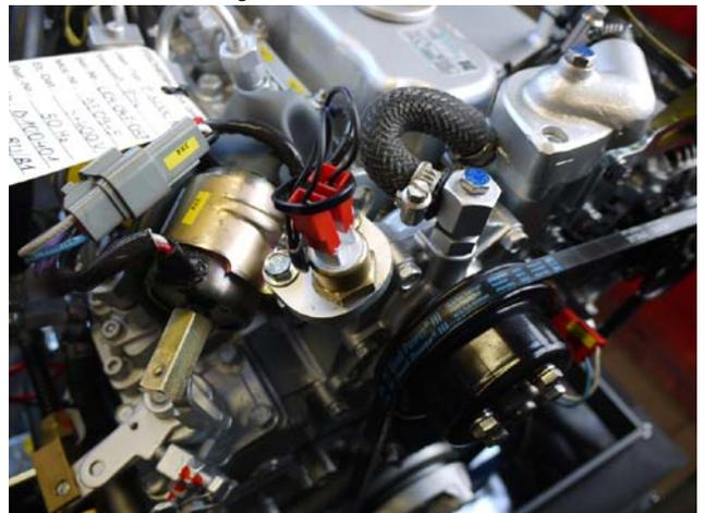
3. Disconnect electric supply line of the thermostat.
