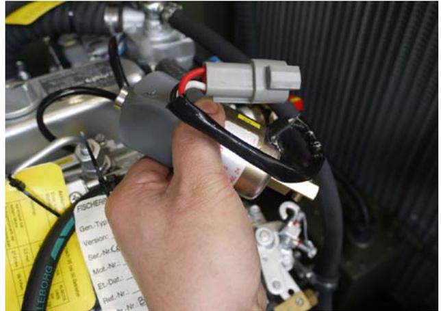
*Fig. 7.28-7: Stop solenoid*
