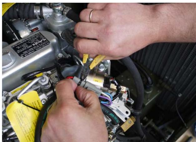
3. Disconnect electric supply line 3X4 from the stop solenoid.
