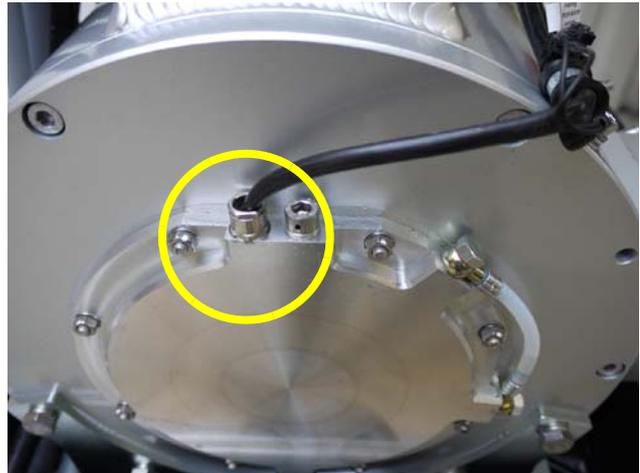
Fig. 4.3.4-4: Thermo-switch at endshield
