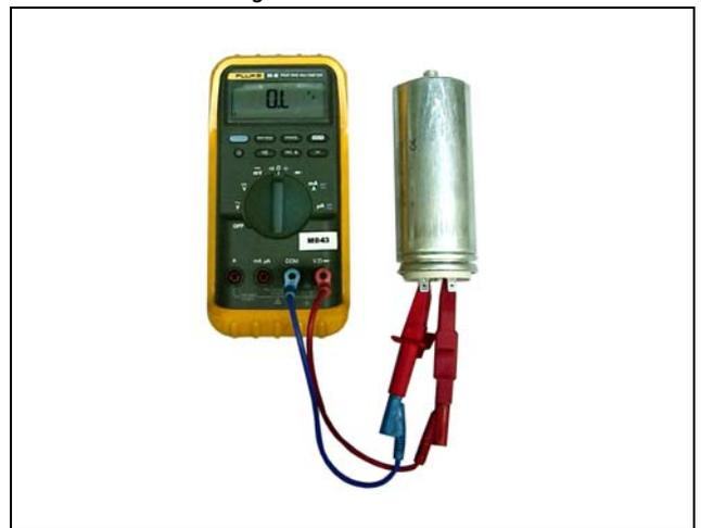
Should a steady sound or no sound be heard, the capacitors are defective and must be replaced.
