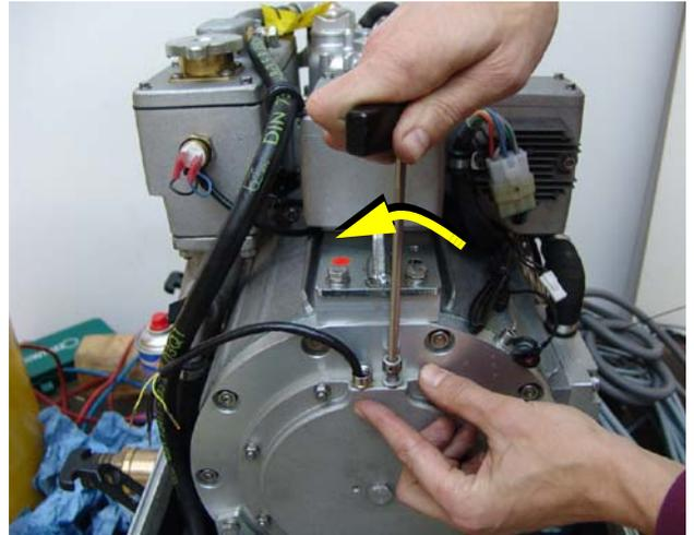
Inserting the hose through the ventilation screws' tap hole.
