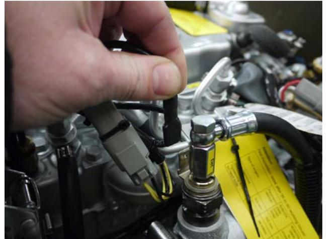
2. A large piece of cloth or absorbent tissue must be placed under the connection to prevent escaping fuel from running into the capsule.
