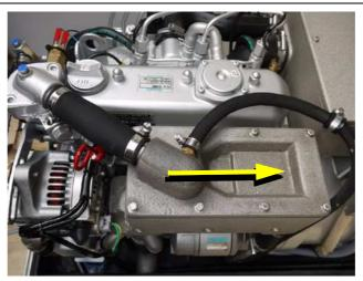
Fig. A.3.3-10: Water-cooled exhaust manifold
