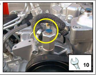
Fig. B.4-2: Ventilating Screw
