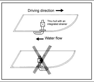
Fig. A.3.2-1: Position of the Thru Hull Fitting
