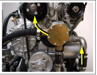
Fig. A.3.3-6: Internal cooling water pump
