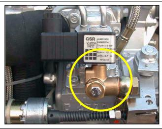
Fig. A.6.5-1: Vent Screw at the Fuel Stop Solenoid Valve
