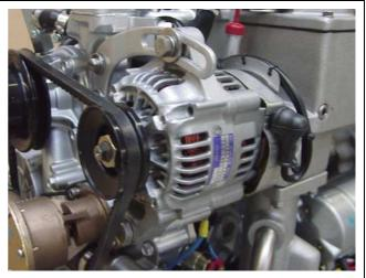
Fig. A.3.6-7: DC-alternator
