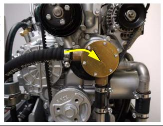
Fig. A.3.2-2: Raw water inpeller pump
