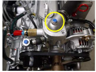
Fig. A.3.3-9: Ventilation screw thermostat housing
