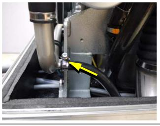
Fig. A.3.3-7: Internal cooling water pump
