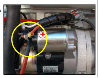
Fig. A.7.1-1: Positive Battery Cable
