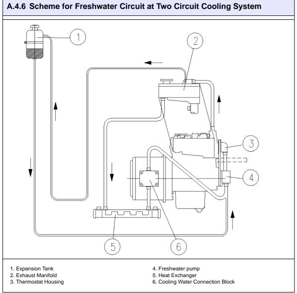
Fig. A-2: Scheme for Freshwater Circuit at Two Circuit Cooling System
