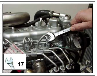
Fig. B.4.1-3: Injection nozzles
