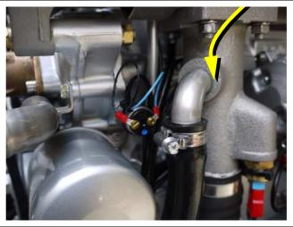
Fig. A.3.5-4: Exhaust elbow
