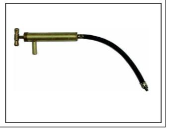
Fig. B.3-3: Oil Drain Pump
