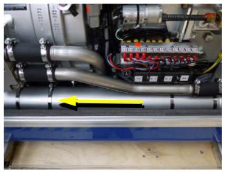
Fig. A.3.2-3: Heat exchanger
