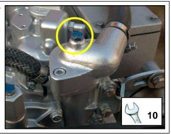
Fig. B.4-3: Ventilating Screw on the Thermostat Housing
