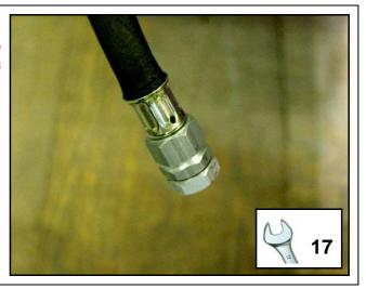
Fig. B.3-2: Oiil Drain Screw
