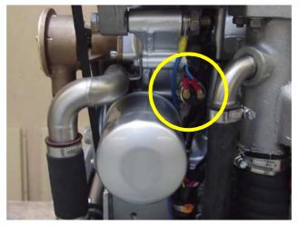
Fig. A.3.7-5: Oil pressure switch
