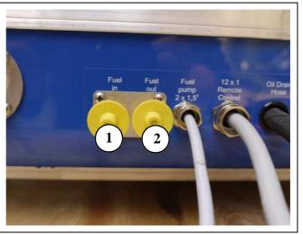
Fig. A.3.4-2: Fuel connections
