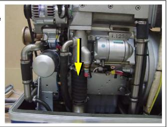
Fig. A.3.5-5: Exhaust connection
