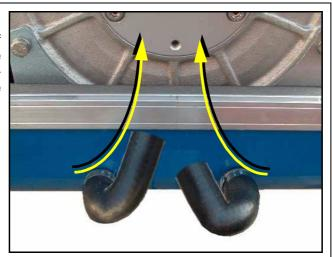
Fig. A.3.5-2: Connection Vent Valve
