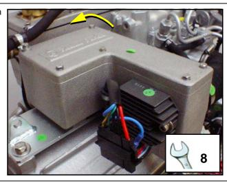
Fig. B.4.3-1: Air Suction Housing
