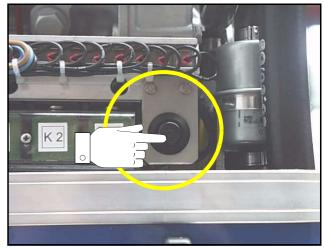
Fig. B.4.1-1: Failure Bypass Switch
