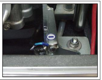
Fig. A.7.1-2: Negative Battery Cable
