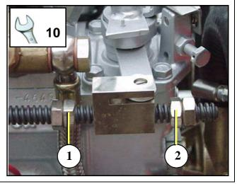
Fig. C.3.2-1: Adjustment Screw Speed Governor
