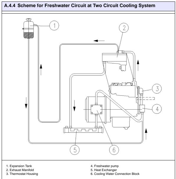
Fig. A-1: Scheme for Freshwater Circuit at Two Circuit Cooling System
