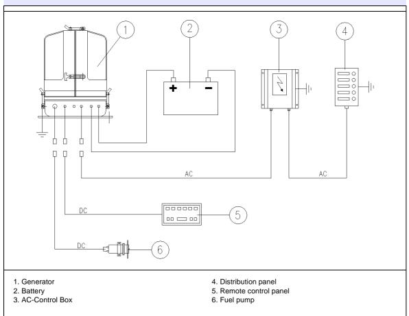
Fig. A.8.1-1: Installation with looped in AC-Control box
