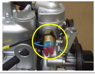
Fig. A.3.7-2: Thermo-switch at thermostat housing
