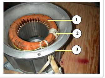
Fig. A.3.7-6: Thermo-switch coil
