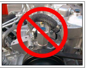
Fig. B.4-5: Ventilation Screw above the Cooling Water Pump Casing
