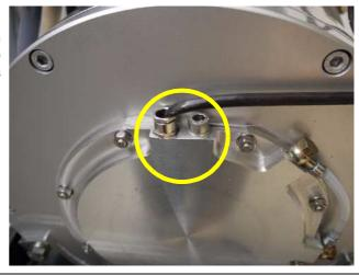
Fig. A.3.7-4: Thermo-switch at endshield
