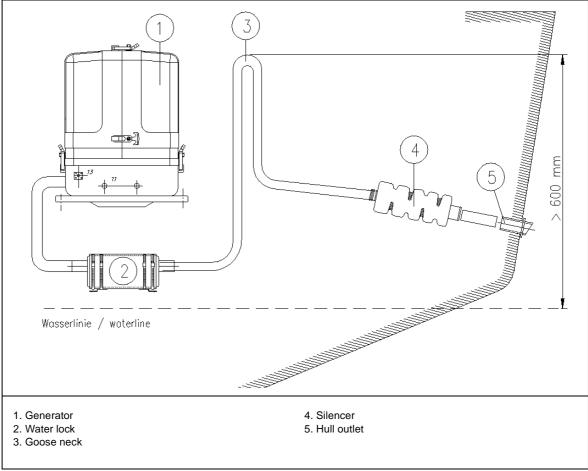
Fig. A.2: Installation Scheme Standard Exhaust System
