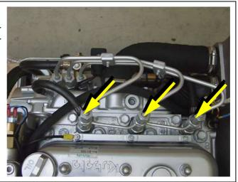
Fig. A.3.4-6: Injection nozzles
