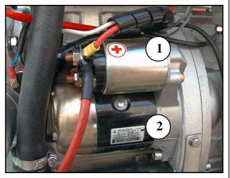
Fig. A.7.1-4: 12 V DC Starter Motor
