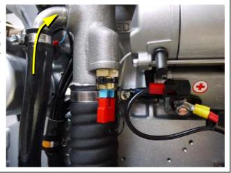
Fig. A.3.2-5: Cooling water injector nozzle
