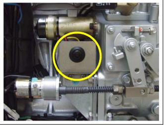
Fig. A.3.7-7: Failure bypass switch
