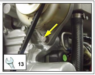
Fig. B.4.5-2: Screw beneath the Alternator
