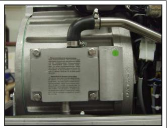
In this case the coolant terminal block is a wearing part. It should always be available in all cases as a spare part on board.
