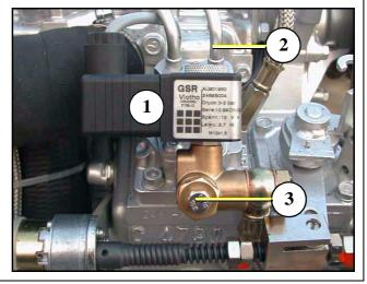
Fig. C.6.1-1: Fuel Solenoid Valve
