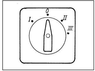
Fig. A.8.2-2: 3-Way Cam Switch
