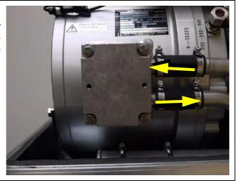
Fig. A.3.3-5: Cooling water connection block
