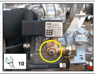
Fig. B.4.1-2: Ventilation Screw at the fuel solenoid valve
