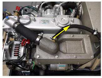
Fig. A.3.3-1: Ventilation pipe
