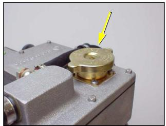
Fig. B.4-4: Colling Water Filler Cap
