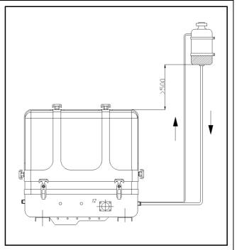
Fig. A.4.1-1: Position of the External Cooling Water Expansion Tank
