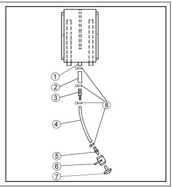
Fig. A.5.2-2: Exhaust Water Separator
