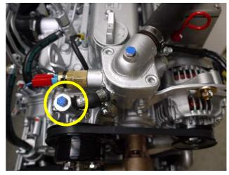
Fig. A.3.3-8: Ventilation screw cooling water pump
