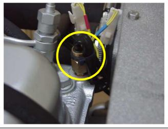
Fig. A.3.7-1: Thermo-switch at cylinder head
