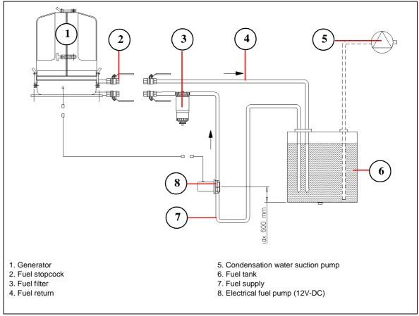
Fig. A.6.1-1: Installation Scheme Fuel System
