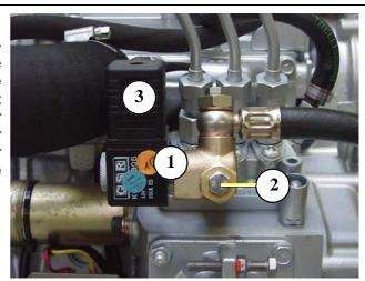
Fig. A.3.4-5: Fuel solenoid valve
