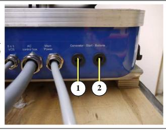
Fig. A.3.6-1: Cable for starter battery
