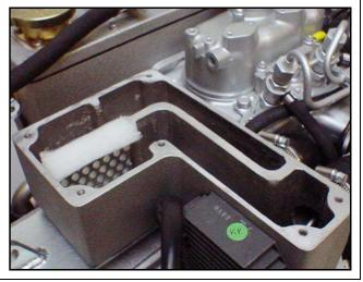
Fig. B.4.3-2: Opened Air Suction Housing
