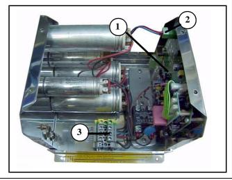
Fig. A.8.3-1: Opened AC Control Box
