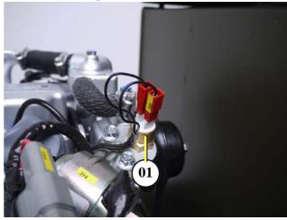
Fig. 6.22-2: Thermocontact
