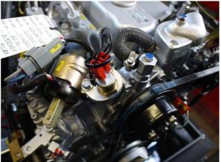
Fig. 6.22-3: Thermocontact
