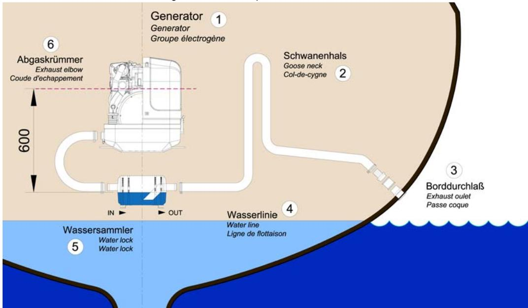
In Fig. 5.7.3.1-1, the waterlock is mounted in center underneath the generator. When the ship tilts, the position of the waterlock related to the critical point at the exhaust hose, changes only slightly.
