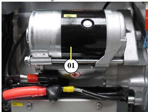
Fig. 7.11-2: Electric starter
