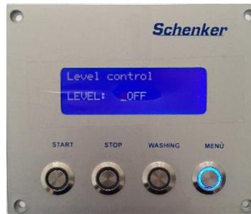
It is an optional function. For activating the automatic start/stop from floating switches select the function Level Control to ON. Then exit from menu pushing STOP.
