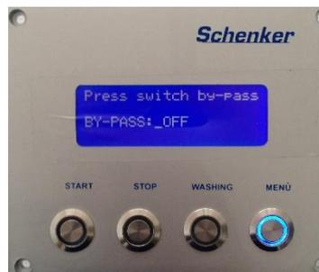
It allows to exclude the sensor (signal pressure switch) that detects the correct cycling of the ERS. The operation with the by-pass is necessary only in case of malfunctioning of the signal pressure switch (in example if the system gets blocks, with the message "SYSTEM BLOCKED", not as consequence of a real hydraulic problem, but just as consequence of the malfunctioning of the probe).
