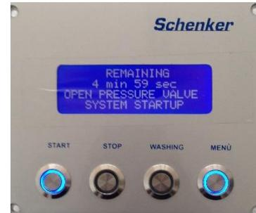
3. The controller starts pump 1 first, and initially the message low pressure will be on. When the pressure will get 2 bars, pump 2 will start automatically (after 5 seconds) and the ERS starts its commutations.
