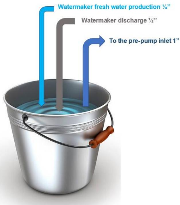
5. Check they are well dipped in the solution and don't inhale air.
