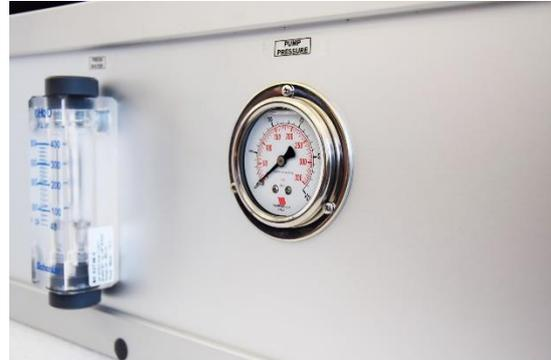
If the average pressure exceeds the above ranges it is necessary to check the membranes cleaning degree. It is necessary to perform the shutdown procedure if the membranes result dirty. If cleaning also results insufficient it could be necessary to perform an alkaline washing using the chemical product SCHENKER CLEANING 2 (SC2). It is recommended to contact a Schenker certified service center.
