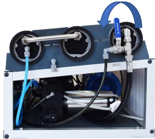
4. Screw the positioner knob clockwise until it can be moved no further. Normally 10 turns at least are needed.
