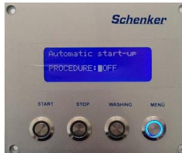
This function activates automatically the first start up procedure. The procedure is necessary when a new machine is started for the first time, or after the filter cartridge replacement, or a general service. The procedure allows to purge completely the air from the system, and from the seawater and the washing fresh water hoses. The depressurization valve must be opened before start the procedure.
