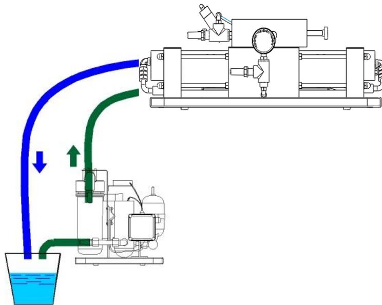
HYDRAULIC SCHEME FOR SHUTDOWN PROCEDURE
