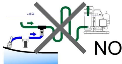
All the hydraulic connections (to exception of the fresh water production) have to be realized with a 16 mm. int. diam. hose and a 1/2" holder. The hydraulic section that is continuously under consistent pressure is the pump outlet – 5 m. filter – watermaker inlet connections. For this section is necessary to use a good quality **PN 16 min.** reinforced hose. An inadequate hose could burst, jeopardizing seriously the safety of the boat.
