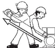
Pull the rope hard and fast. Pull it all the way out. Use two hands if necessary.
